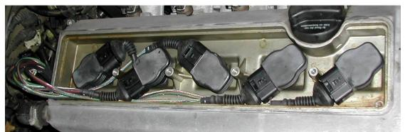
6) Plug in the two 3-pin connectors to the factory harness, it doesn't matter which connector gets plugged in to which female 3-pin. These are just the coil power leads.
