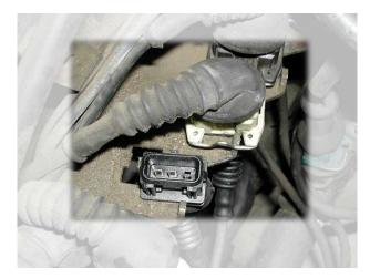
7) Plug in the two 4-pin connectors to the factory harness. Take note that you are plugging them in correctly. You will notice that one connector has 4 male pins, the other has only 2. Make sure the 4-pinned connector gets plugged into the brown/fully populated connector. The other with the missing pins gets plugged into the black female connector with 3 pins.
