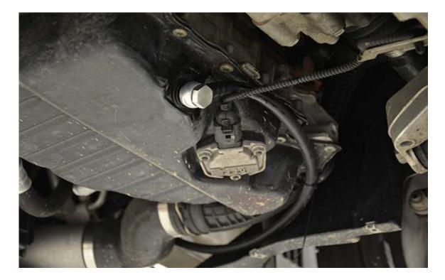
**Step 5** – Fill the vehicle with the appropriate amount of oil. Trim any zip-ties. Make sure than all lines are secured properly and routed correctly.
