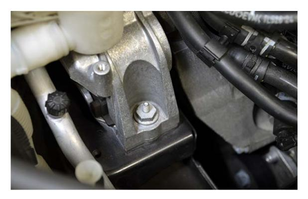
**Step 11** – Mount the catch can to the passenger side engine mount using the supplied bolt. **Please Note: If you are** installing the optional oil drain kit, skip ahead to the instructions for installing the oil drain kit before mounting the catch can.
