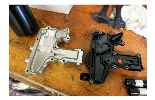
**Step 7** – Position the 034Motorsport Valve Cover Breather Adapter such that the holes align with the threaded holes in the valve cover, and push the PCV assembly to compressor inlet tube into it until it seats.
