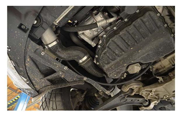
**Step 3** – Drain your oil by removing the factory oil drain plug. If you drain it into a clean pan, it can be reused. If you do not wish to reuse it, you can perform an oil change at this time.
