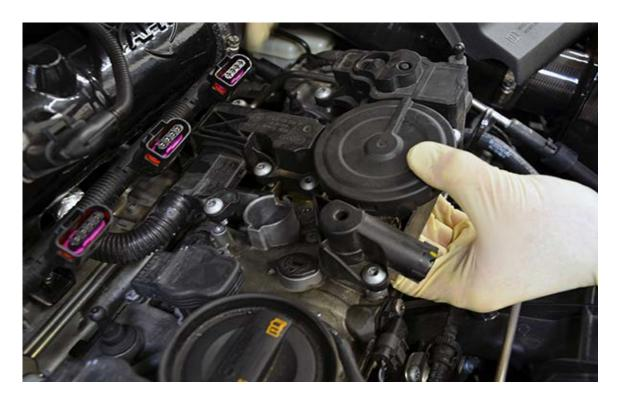
**Step 6** – Remove the factory rubber seal from the PCV assembly, and install it into the Valve Cover Breather Adapter.
