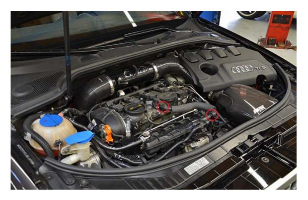
**Step 3** – Install the 2.0 TSI Intake Manifold Plug to black off the port where the valve cover breather to intake manifold hose was. Rotate the locking tab down to secure the plug against the plastic rib on the intake manifold plenum. *If you intend to use this as a boost tap, unscrew the 1/8" NPT Plug, and replace it with a 1/8" NPT to appropriate barbed brass fitting for use with your boost gauge's vacuum line.*
