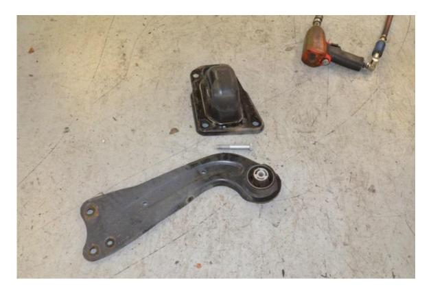
**Step 11** – Install supplied spacers into spherical trailing arm bearing.
