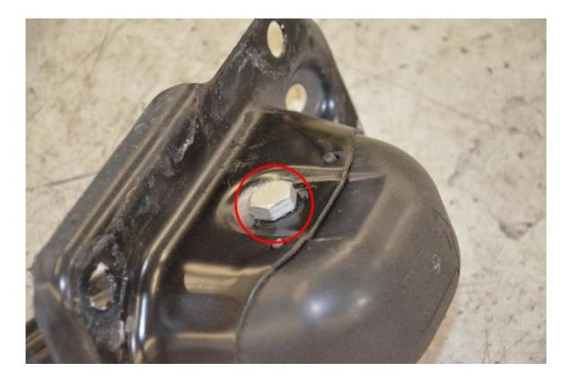
**Step 10** – Trailing arm and housing should be separated now. Discard old trailing arm, and identify correct replacement from 034Motorsport Spherical Rear Trailing Arm Pair.
