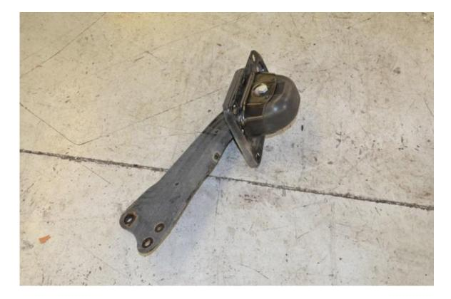
Step 9 – Remove 18mm bolt holding housing to trailing arm, and remove housing.
