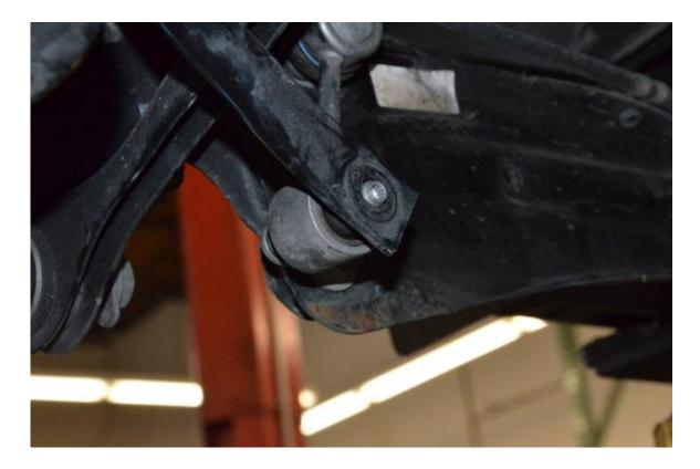
**Step 5** – Remove the two 18mm bolts holding trailing arm to upright.
