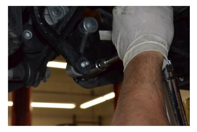
**Step 16** – Reinstall parking brake cable retaining clip with T30 screw torqued to **8 Nm**.
