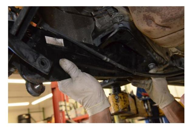
**Step 14** – Tighten 4 16mm bolts holding housing to chassis to **50 Nm + 45 degrees**.
