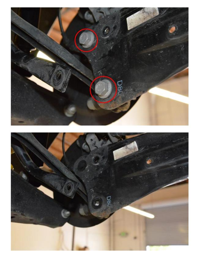
**Step 6** – Remove the four 16mm bolts holding the trailing arm housing to the chassis.
