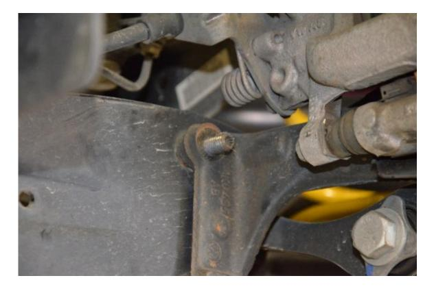
**Step 4** – Remove 16mm nuts holding the rear sway bar end link to the sway bar. A 6mm triple square can be used to prevent the threaded inner from turning. Remove the end link.
