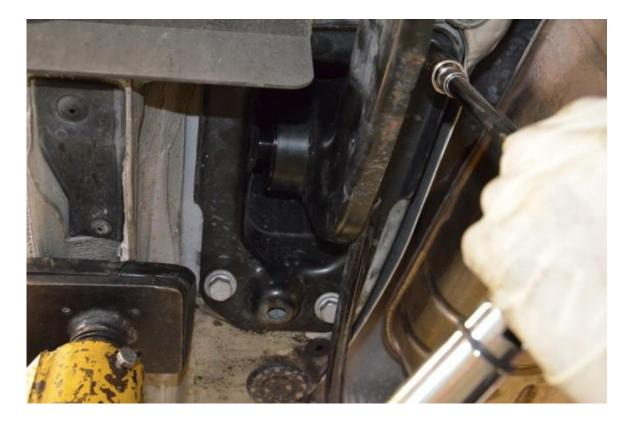
Step 15 – Tighten 2 18mm bolts holding arm to upright to 90 Nm.
