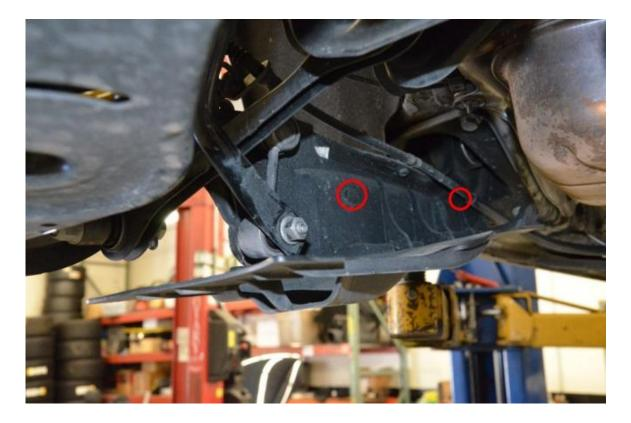
**Step 3** – Remove 16mm nut holding rear sway bar end links to trailing arm.
