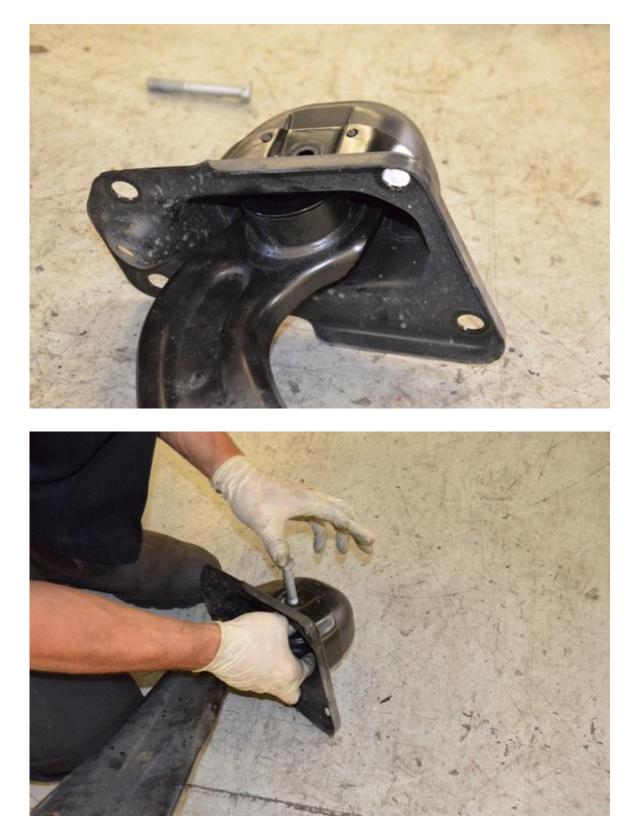
**Step 13** – Begin to reinstall arm and housing assembly into the vehicle. Use one bolt at each end to line up. You may have to push up on the upright and/or compress the suspension slightly to align all holes.
