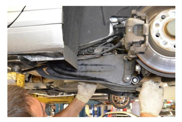
**Step 19** – We strongly recommend having the rear suspension aligned to factory specifications immediately after installing the 034Motorsport Rear Trailing Arm Spherical Bearing Upgrade Kit.
