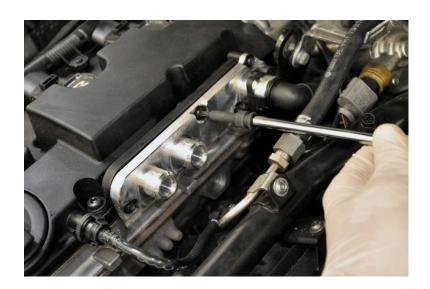
**Step 13** – Route the Silicone Breather Hoses as pictured below, and secure to the Valve Cover Breather Adapter and Catch Can with the supplied Hose Clamps.
