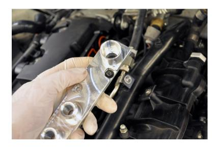
**Step 11** – Attach the factory block breather hose to the Valve Cover Breather Adapter by pressing it firmly over the nipple until it locks into place.
