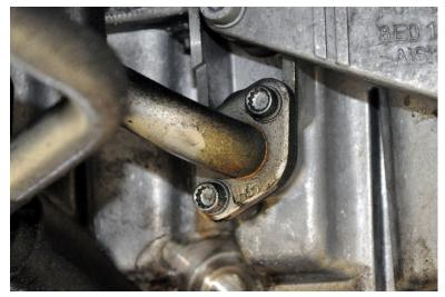
**Step 16** – Install the Catch Can Oil Drain Adapter Kit as pictured below, with the NPT fitting installed using Thread Sealant and oriented such that the barbed brass nipple is facing up. Secure using the supplied M6x50 Bolt, with one gasket on each side of the billet aluminum adapter.
