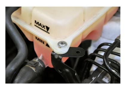
**Step 4** – Position the Catch Can such that the holes on the Mounting Bracket align with the holes on the top and side of the factory coolant reservoir bracket. Secure to the side of the factory bracket using the supplied M6x25 Bolt, M6 Washers, and M6 Nut.
