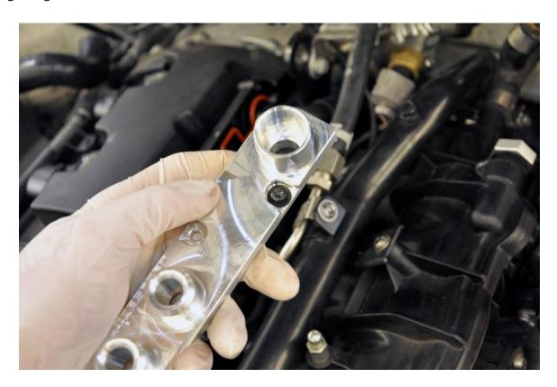
**Step 11** – Attach the factory block breather hose to the Valve Cover Breather Adapter by pressing it firmly over the nipple until it locks into place.
