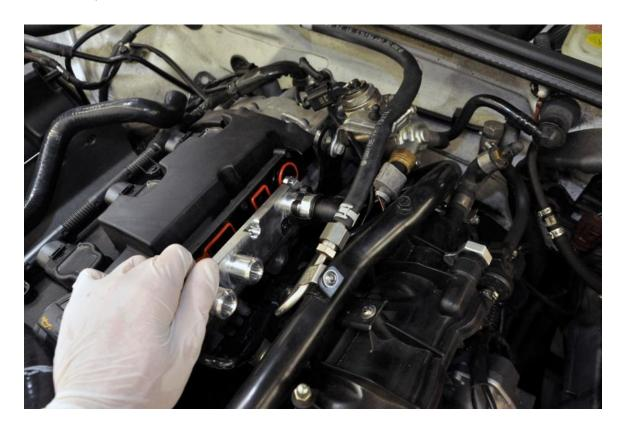
**Step 12** – Secure the Valve Cover Breather Adapter to the valve cover using the factory T25 Torx screws. **DO NOT OVER- TIGHTEN THESE SCREWS! THE OEM VALVE COVER IS PLASTIC AND CAN STRIP EASILY!**
