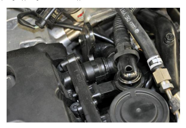
**Step 9** – Remove the 4 T25 Torx screws securing the factory PCV check valve assembly to the valve cover. *Be careful to avoid dropping any screws into the ports in the valve cover.*
