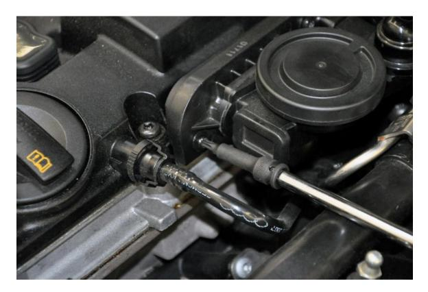
**Step 10** – Slide the bottom Torx screw into the 034Motorsport B7 Audi A4 2.0T FSI Valve Cover Breather Adapter before attempting to align it with the valve cover.
