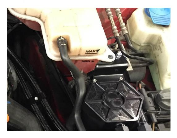
**Step 5** – Realign the coolant reservoir over the top of the Mounting Bracket and reinstall the factory phillips-head screw.
