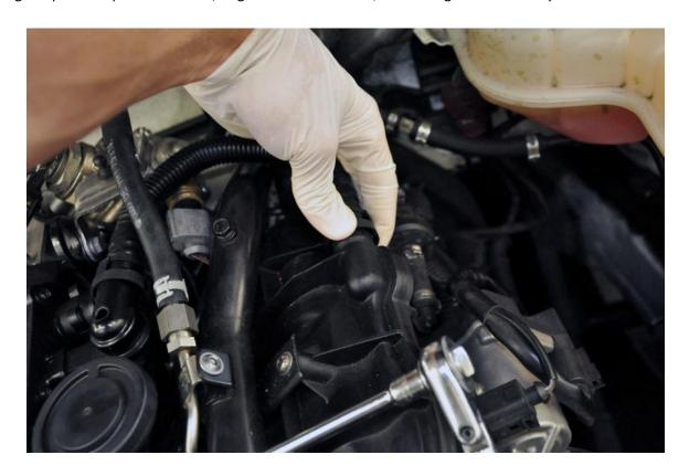
**Step 7** – Install the B7 Audi A4 2.0T FSI Intake Manifold Plug to black off the port where the valve cover breather to intake manifold hose was. Rotate the locking tab down to secure the plug against the plastic rib on the intake manifold plenum. If you intend to use this as a boost tap, unscrew the 1/8" NPT Plug, and replace it with a 1/8" NPT to appropriate barbed brass fitting for use with your boost gauge's vacuum line.
