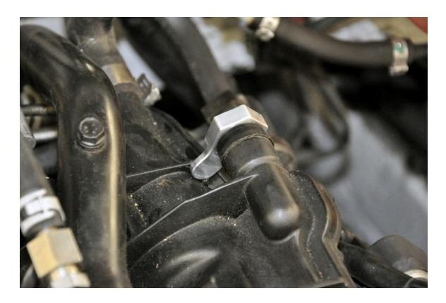
**Step 8** – Locate and detach the factory block breather hose from the valve cover breather. Detach by carefully pulling up on the clip and gently pushing the hose off of the nipple.
