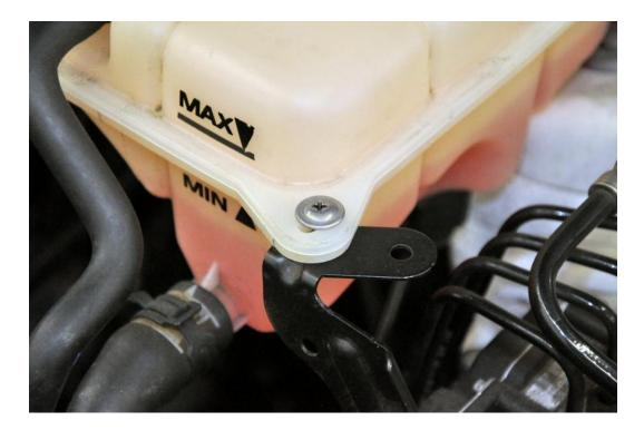
**Step 4** – Position the Catch Can such that the holes on the Mounting Bracket align with the holes on the top and side of the factory coolant reservoir bracket. Secure to the second bolt hole on top of the factory bracket using the supplied M6x25 Bolt, M6 Washers, and M6 Nut.
