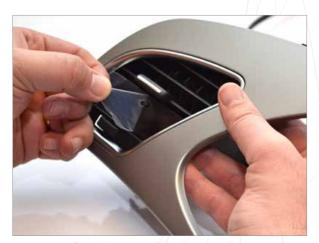
Peel the remaining protective covering off the gauge and it is ready to go back into the car. Follow the generic "in car" instructions for the remainder of the install.
