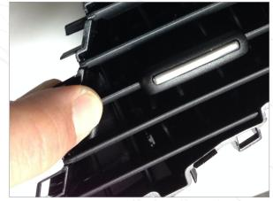
Place index finger over the central control slat while removing lower slats. This will insure control and up slats remain in the vent and in union with one another.
