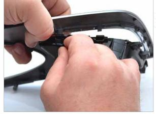
Using a flat blade screwdriver, unclip the trim from the vent, be careful that the slats do not fall out.
