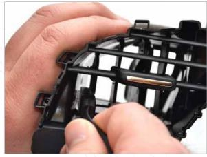
Insert the wire in the vent by squeezing the connector through the left bottom corner as shown. Feed all the wire through.
