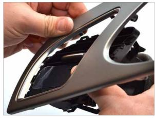
Carefully re-attach the trim to the vent assembly. If you have trouble keeping the parts from falling out, you can use a temporary piece of tape across the right side to hold them in until the trim is in place.
