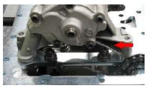
14.) Once the outer oil pan is reinforced, machine cut two grooves to clear the girdle nuts.
