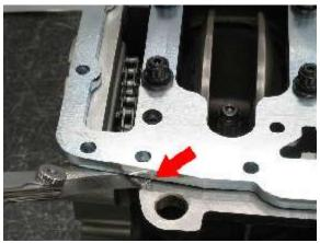
10.) After the main bearing girdle has been installed, fit the oil pump to the block. A section of the pump may not clear the nut and will have to be cut (06A). Mark the section with a permanent marker and machine as necessary.
