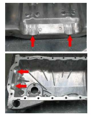
15.) Apply silicone sealant to the oil pan and install. Torque the bolts in the sequence and specification provided by the factory.
