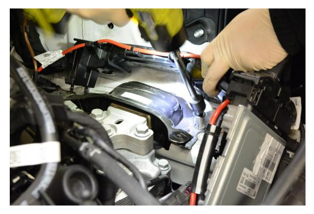
**Step 24** – Using an 18mm socket, remove the three bolts securing the Transmission Mount to the transmission.
