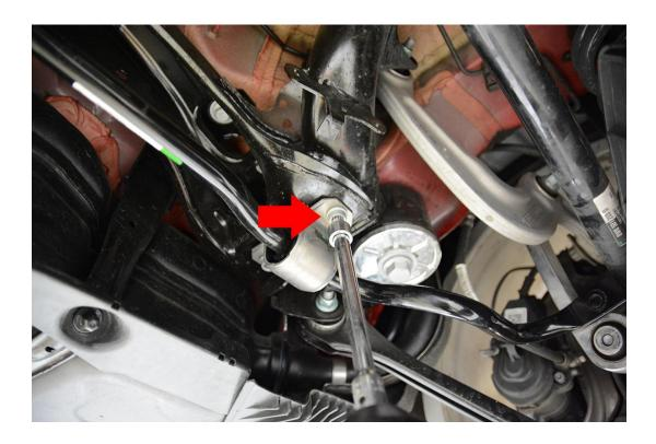
**Step 4** – With the sway bar mounting brackets and end links removed, snake out the rear sway bar from underneath the vehicle.
