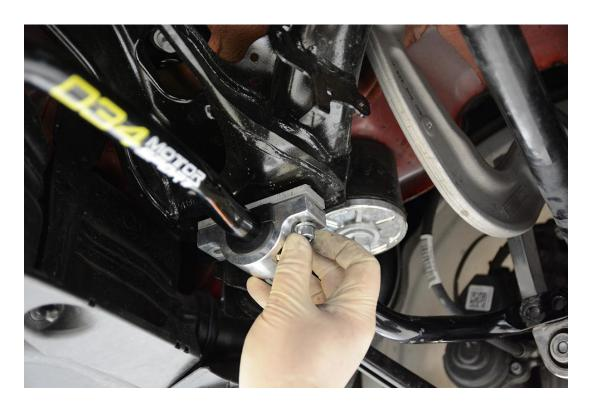
**Step 8** – Attach the sway bar end links to the 034Motorsport Dynamic+ Adjustable Rear Sway Bar using the factory hardware. Torque to 40 Nm + 180 Degrees.
