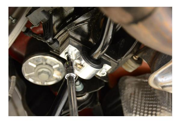
**Step 10** – Raise the exhaust and reinstall the exhaust hanger bolts you removed in Step 1.
