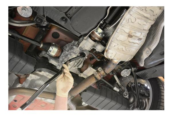
**Step 5** – After applying the supplied grease on the inside of the bushings, install the polyurethane sway bar bushings and billet aluminum brackets onto the bar as shown.
