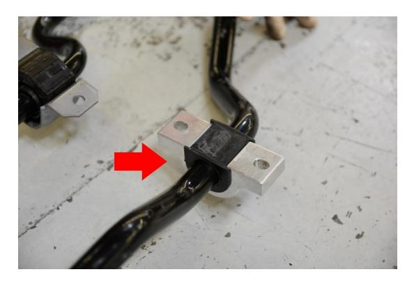
**Step 6** – Install the 034Motorsport Dynamic+ Adjustable Rear Sway Bar in the same orientation as the factory bar, placing the supplied Sway Bar Bushing Backing Plates between the bushing/bracket and subframe as shown below.
