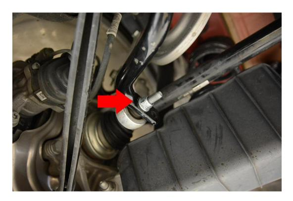
**Step 9** – Tighten the sway bar mount bracket bolts to 28 Nm.
