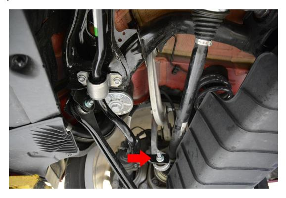
**Step 3** – Remove the triple square bolts securing the factory sway bar mounting brackets to the rear subframe.
