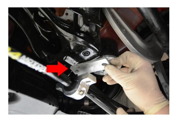
**Step 7** –Snug up the supplied Sway Bar Bracket hardware, but do not tighten fully.
