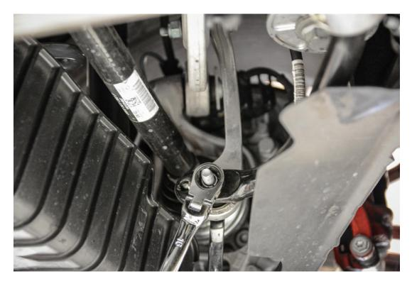
**Step 3** – With the same 2 16mm wrenches, loosen and remove the upper nut securing the sway bar end link to the rear control arm.
