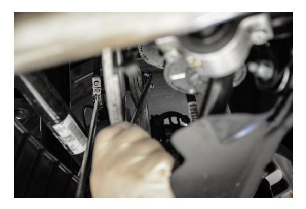
**Step 4** – Remove the lower bolt front the bottom of the rear sway bar end link and set to the side. This will be needed when installing the 034Motorsport Adjustable Rear Sway Bar End Link.
