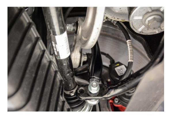
**Step 10** – Using 2 16mm wrenches, tighten the 034Motorsport Adjustable Rear End Link to the rear sway bar. Torque to **40Nm + 180 Degrees.**
