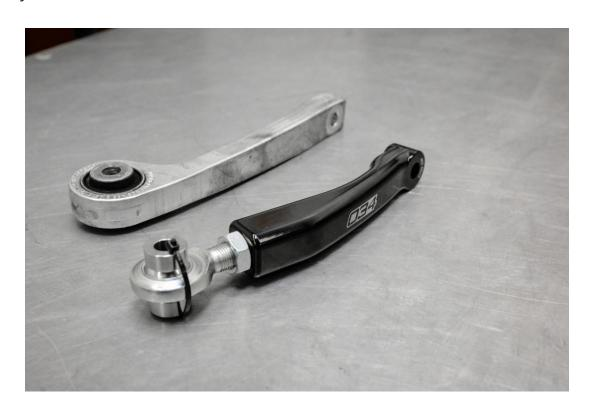
**Step 7** –Orient the 034Motorsport Adjustable Rear Sway Bar End Link so that the logo faces forward, and the heim joint and spacers are on the bottom. Pre-install factory upper end link bolt through the 034Motorsport Adjustable Rear Sway Bar End Link, orienting the bolt from the front of the vehicle to the back.
