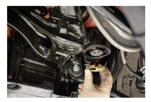
**Step 8** –The front subframe bushing should be fully exposed and resemble the picture below.
