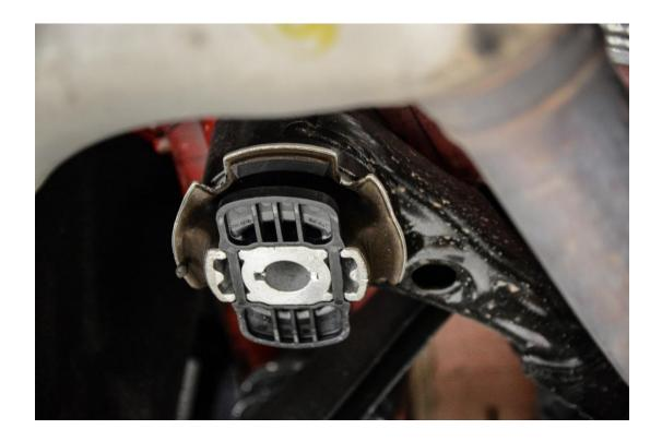
**Step 15 –** The rear bushing of the rear subframe should resemble the photo below.
