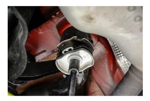
**Step 13** – With a pry bar, remove the factory metal retainer from the rubber bushing.
