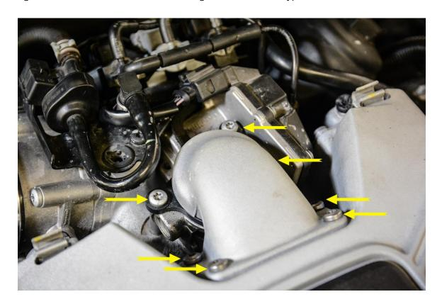
**Step 4** – At this point, 7 bolts should have been removed and the elbow will be free. Lift up to remove elbow from engine.
