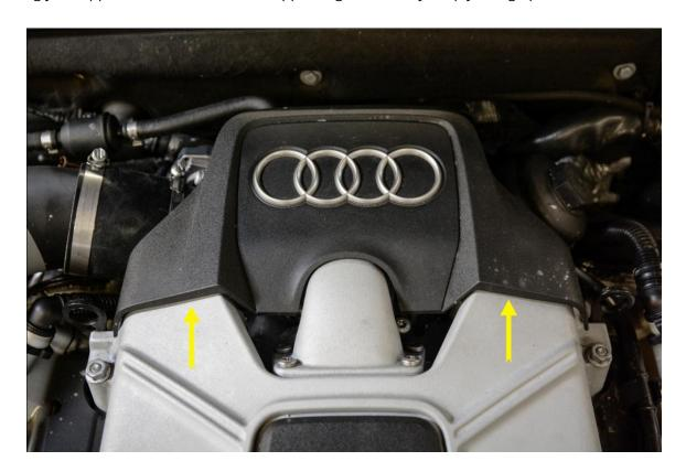
**Step 2** – Using a T30 Torx, remove the 4 Bolts securing the elbow to the supercharger.
