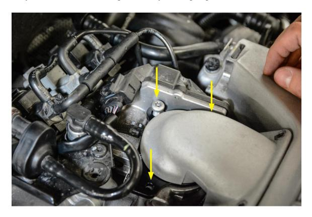
**Step 11** – Secure elbow to supercharger using remaining 4 factory bolts and tighten using a T30 Torx.
