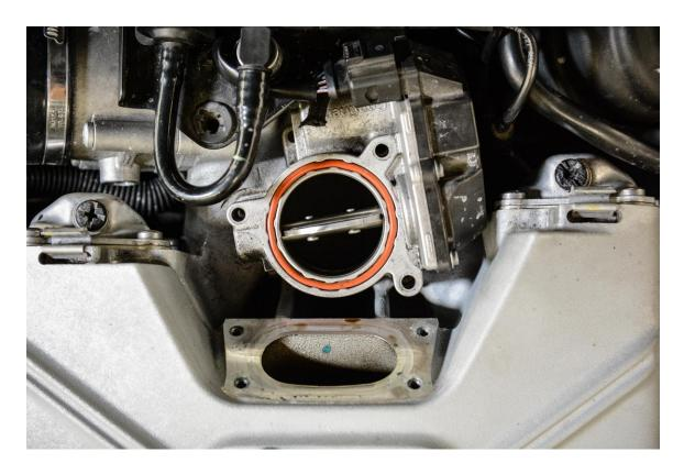
**Step 7** – Using a Small Pry Bar or Flat Head Screwdriver, remove factory plastic plate from the elbow.
