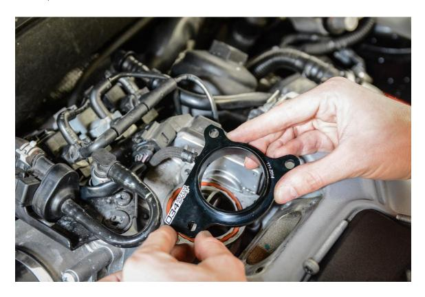
**Step 9** – Place 034Motorsport Boost Tap on top of bypass valve, and align bolt holes.
