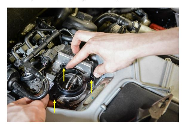
**Step 10** – Place elbow over lip on 034Motorsport Boost Tap and secure 034motorsport Boost Tap to bypass valve with the 3 factory bolts. Use a T30 Torx to snug the 3 factory bolts finger tight.
