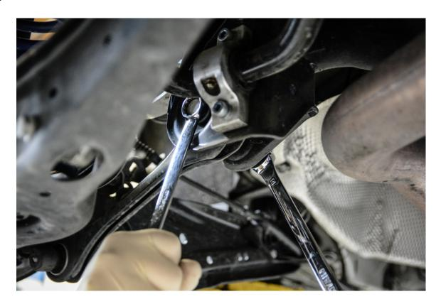
**Step 7** – With a pry bar, dislodge the rear too link from the rear hub assembly.
