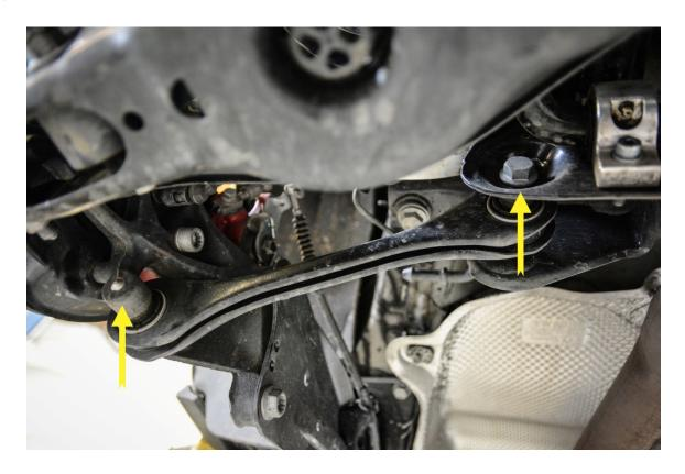
**Step 5** – Using an 18mm wrench or socket, remove the outer bolt securing the toe link to the hub assembly.
