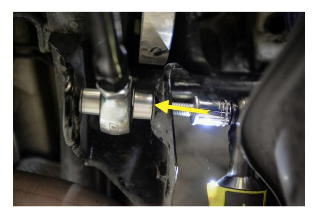
**Step 14 –** Reinstall the lower rear sway bar end link bolt, securing the rear sway bar end link to the lower rear control arm. Torque to **35 Nm**.
