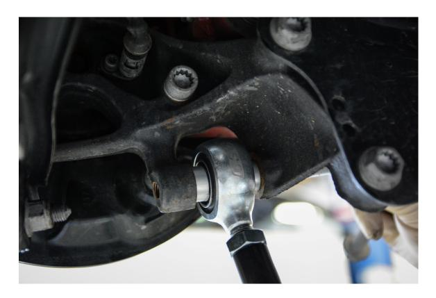
**Step 11** – Install the factory outer toe link bolt, securing the 034Motorsport Density Line Adjustable Rear Toe Link to the rear hub assembly. Leave a little loose for now.
