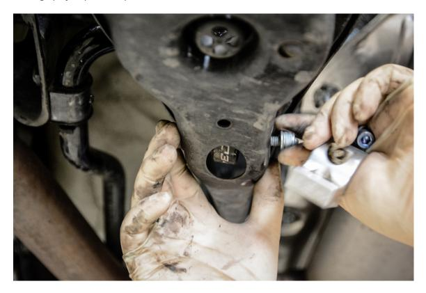
**Step 4** – Locate the 2 bolts (inner and outer) securing the factory rear toe link to the rear subframe and rear hub assembly.
