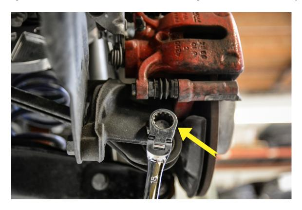
**Step 6** – Using a pair of 18mm wrenches (or 18mm socket & 18mm wrench), remove the factory nut and bolt securing the toe link to the rear subframe.
