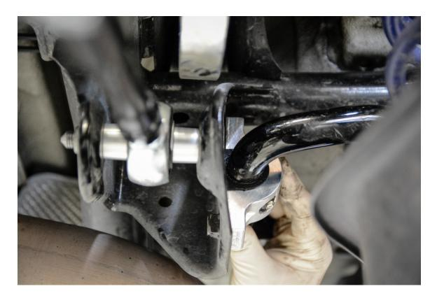
**Step 16 –** Double check the installation, and verify that all swaybar connections are torqued to spec. Either use pole jacks to lift the rear suspension, or use an alignment rack or service pit to torque the inner and outer toe link bolts on both sides. **NOTE:** the suspension **MUST** be at static ride height before tightening/torquing these bolts to avoid bushing damage. Torque inner and outer toe link bolts to **70NM + 180 degrees**.
