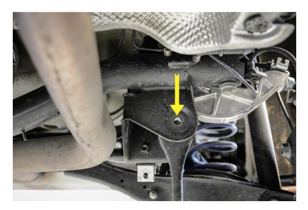
**Step 9** – Set the new 034Motorsport Density Line Adjustable Rear Toe Link to the same length as the factory toe link by aligning the bolts through both the factory and 034Motorsport rear toe links simultaneously.
