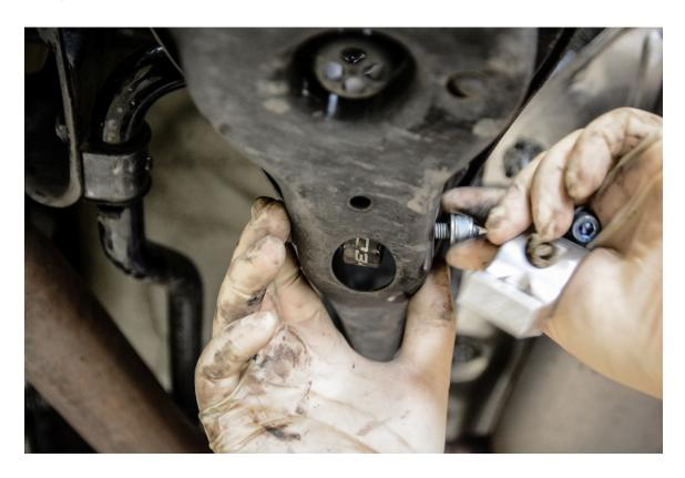
**Step 15 –** Reinstall rear swaybar mounting brackets with existing bolts. Torque to **28 Nm**.
