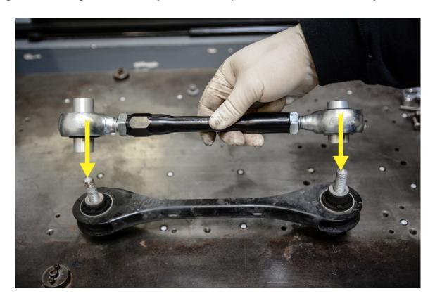
**Step 10** – Align the bolt holes of 034Motorsport Density Line Adjustable Rear Toe Link with the rear hub assembly. **Note:** Position such that the short spacers are on the outside (hub assembly) and taller spacers mount to the rear subframe.
