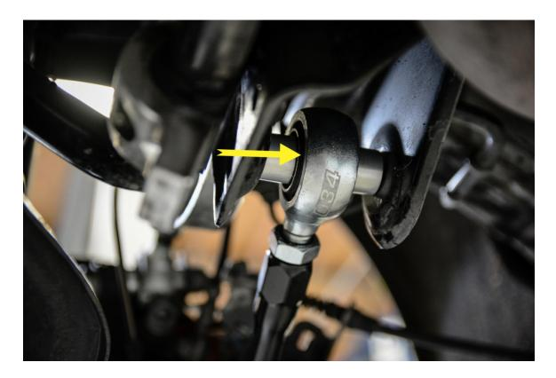
**Step 13 –** With the bolt holes aligned, install the factory inner toe link bolt using an 18mm socket, securing the 034Motorsport Density Line Adjustable Rear Toe Link to the rear subframe. Leave a little loose for now.
