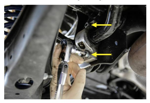
**Step 3** – Remove the lower rear sway bar end link bolt from the lower control arm. By doing this, the rear sway bar should have enough play to provide space for inner toe link bolt removal.
