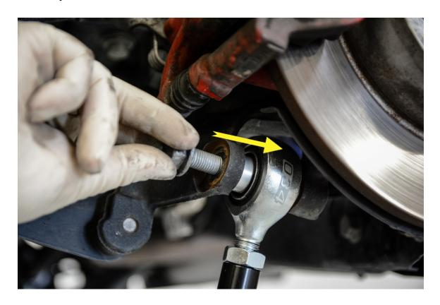
**Step 12 –** Position the inner rod end within the rear subframe provisions and align bolt holes.
