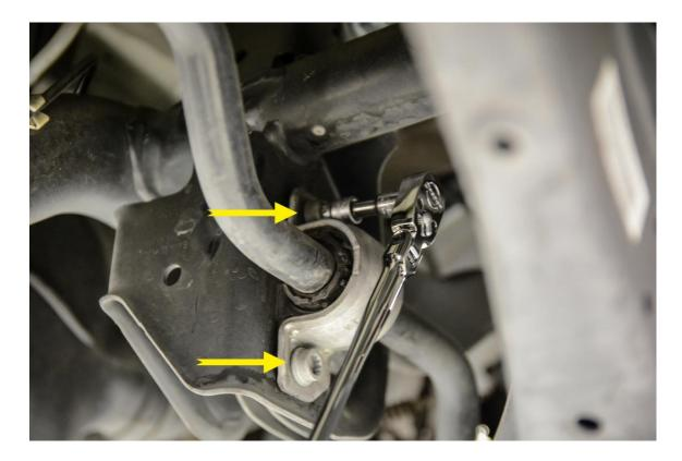
**Step 5** –Remove the factory sway bar from the car, careful to rotate it around the exhaust. install the 034Motorsport Solid Rear Sway Bar.
