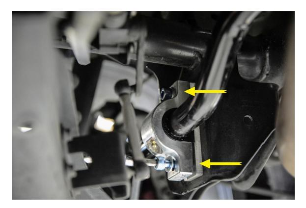
**Step 10** – With the sway bar in place, install the supplied M10x65 bolts and nylock nuts to the factory rear end links using a 15mm and 16mm wrench. Torque the stock hardware to 35 Nm.
