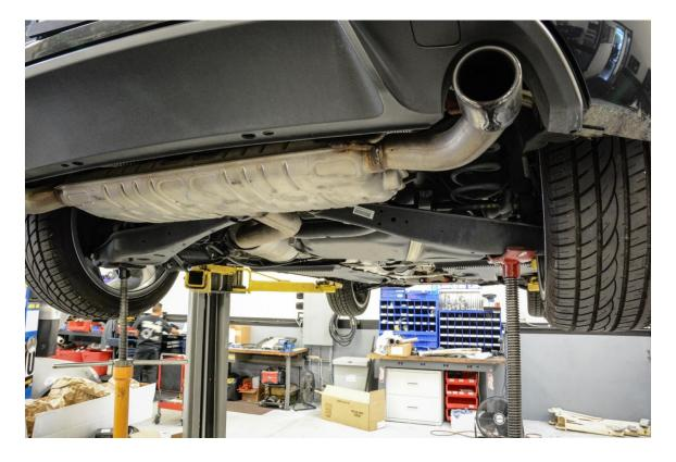
**Step 2** – Using a 16mm wrench and 6mm triple square, remove the nut securing each of the rear sway bar end links to the rear sway bar.
