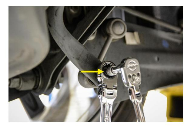
**Step 3** – Once the nut is free from each of the sway bar end links, rotate the sway bar so that it is free from each end link.
