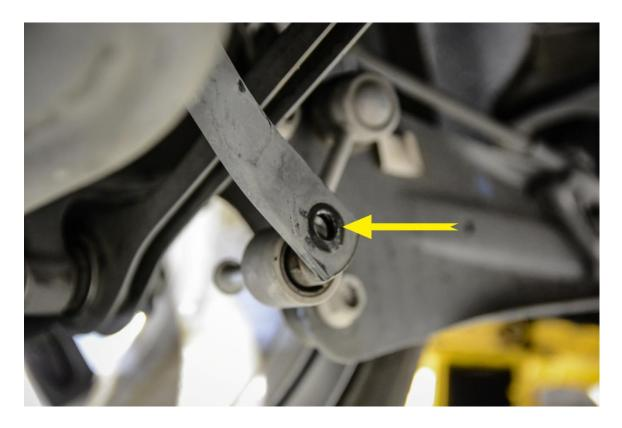
**Step 4** – Using the 10mm Triple Square, remove the two M8 Bolts securing each of the factory rear sway bar mounting brackets to the subframe.
