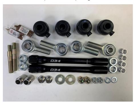
**Step B**Apply half packet of anti-seize to each rod end
