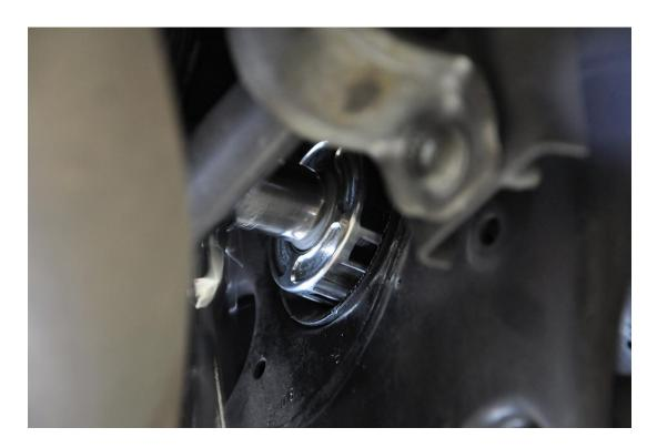
**Step 10** – When tightening, make sure that the bolt head fits into the machined locating recess in the Differential Carrier Mount Insert, as pictured below.
