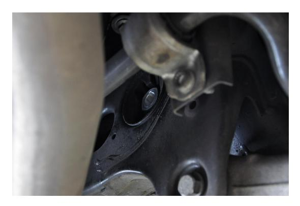
**Step 5** – Spray some silicone lubricant into the voids in the rear differential carrier mount. This will help make insertion of the insert into your car's undercarriage more pleasurable for both you and your vehicle.
