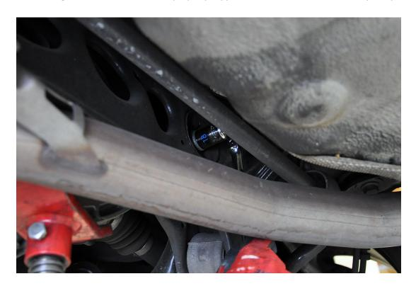
**Step 4** – Observe the rear differential carrier mount, and take note of the large voids in the rubber. They are there to limit NVH transfer into the cabin, but also allow for performance-hindering drivetrain slop. These voids are what the Rear Differential Carrier Mount Insert Kit is designed to fill, reducing unwanted twist in the rear differential mount.
