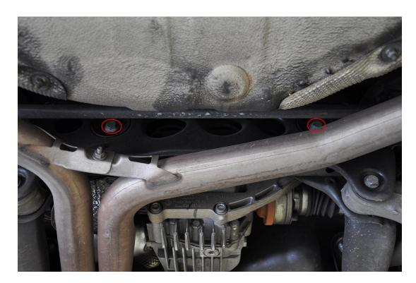
**Step 2** — Pick a side to start on — left or right: you can choose your own adventure! — and support the rear differential carrier using a jack, or transmission jack, or your friend who works out a lot, named Jack. The differential must be properly supported before any bolts are removed, or else gravity will cause it to swing down and bap you on the noggin.
