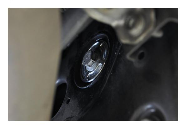
**Step 11** – Repeat the installation process on the other side of the rear differential carrier. You may need to move the jack, transmission jack, or your friend named Jack to better support the other side of the rear differential carrier.
