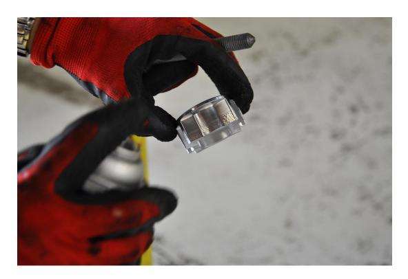
**Step 7** – Slip the shiny new 034Motorsport Differential Carrier Mount Insert into the void of the factory mount. The 034 logos should be rotated to the top/bottom to ensure that the insert lines up with the voids in the mount, as pictured below. If it doesn't feel right the first time, pull it out, and then stick it back in. Repeat as necessary until satisfied.
