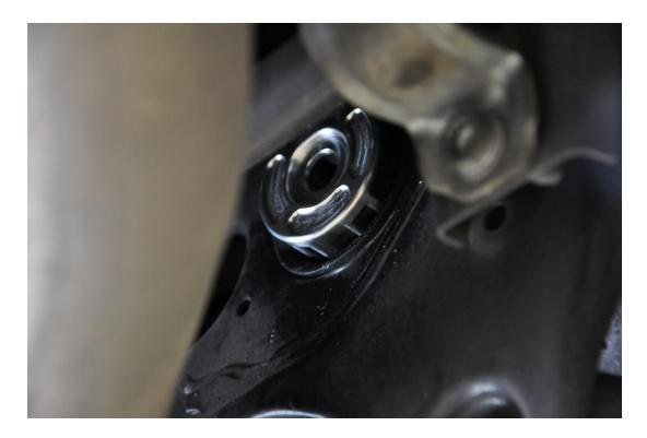
**Step 8** – Secure the 034Motorsport Differential Carrier Mount Insert using the 18mm hex head bolt you loosened in Step 3.
