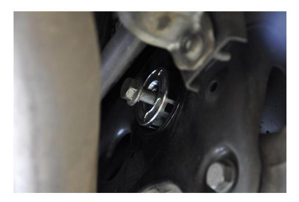
**Step 9** – Torque the crossmember to rear differential carrier bolt to 55 Nm using a torque wrench. Do not overtighten the bolt!
