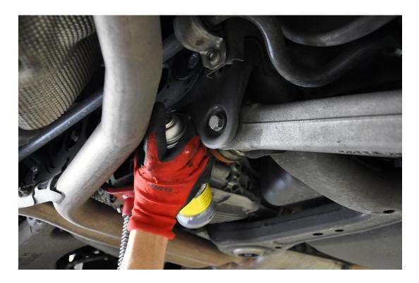
**Step 6** – For good measure, spray some extra silicone lubricant on the mating surfaces of the 034Motorsport Rear Differential Carrier Insert itself.
