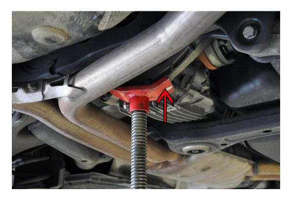
**Step 3** – Using the 18mm socket and your superhuman strength, loosen the hex head bolt going through the rear differential carrier bushing. Make sure the carrier is properly supported, and remove the bolt completely.
