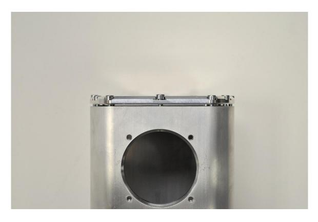
**Step 5** – Apply a thin layer of the supplied RTV to the SRI Throttle Body Elbow as pictured below.
