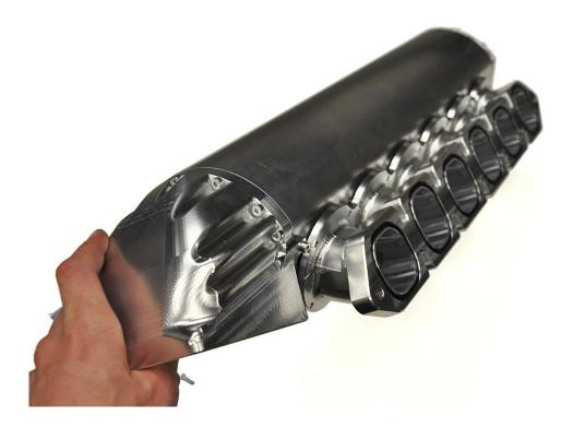
**Step 8** – Lubricating the six o-rings on the plenum side of the SRI Runners will help with this step. Secure the SRI Runners to the SRI Plenum using the twenty-four M4 x 12mm hex bolts with Blue Loctite. Torque bolts to 5 Nm.
