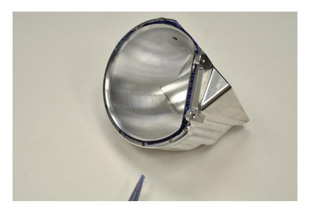
**Step 6** – Using the nine M4 x 16mm allen bolts and Blue Loctite, attach the SRI Throttle Body Elbow to the SRI Plenum. The flat mating surface for the throttle body will line up with the notch in the SRI Plenum. Install the two remaining M4 x 12mm allen bolts with Blue Loctite in the two holes on the Throttle Body Elbow to the flat side of the SRI Plenum. Torque all bolts to 5 Nm.
