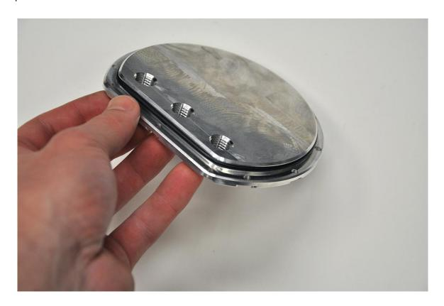
**Step 2** – Locate the six 44mm x 3.5mm o-rings and the SRI runners. These o-rings are visually thicker than the 45mm x 3mm ones. Do not get them confused! The six 44mm x 3.5mm o-rings install into the receiver grooves located on the plenum side of the runners, as pictured below.
