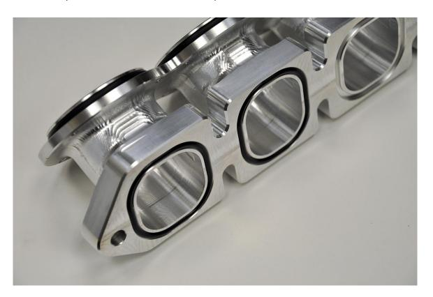
**Step 4** – Using twelve of the shorter M4 x 12mm allen bolts and Blue Loctite, install the SRI End Plate onto the side of the SRI Plenum that *does not* have a notch for the throttle body. Make sure not to pinch the o-ring! Lubricating the oring helps with this step, and the bolts can be used to *carefully* pull the end plate to the plenum. Torque bolts to 5 Nm.
