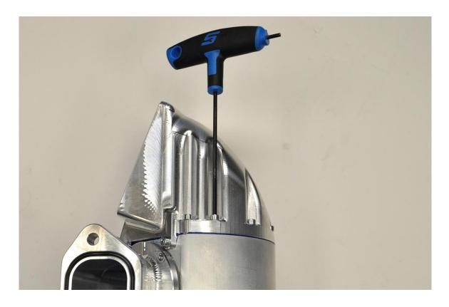
**Step 7** – Attach the SRI Runners to the SRI Plenum as pictured below. The orientation is important!
