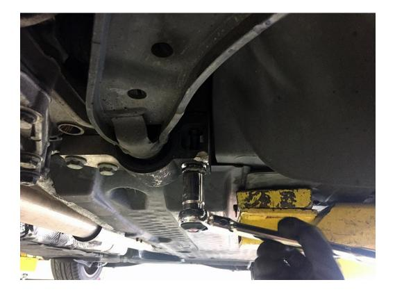
**Step 5** – Note the installation orientation of the locking collars as shown below. The top collars have prominent subframe locating features at the top, while the bottom ones have flat surfaces for the shouldered M12 bolts.
