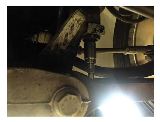
**Step 12** – At this point, you should be a pro at installing the locking collars in the correct orientation, so keep doing what you have been for the last four, and thread in the supplied M12x90mm bolts when you're done.
