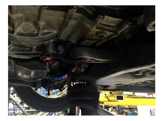
**Step 3** – Loosen the 16 bolts circled below using 13mm, 16mm, and 18mm sockets. 4-5 counterclockwise turns should be enough to allow the subframe to shift for centering. This step can be performed with or without a breaker bar to tailor the resistance to your level of strength conditioning. We recommend a 45-60 second rest every 4 bolts.
