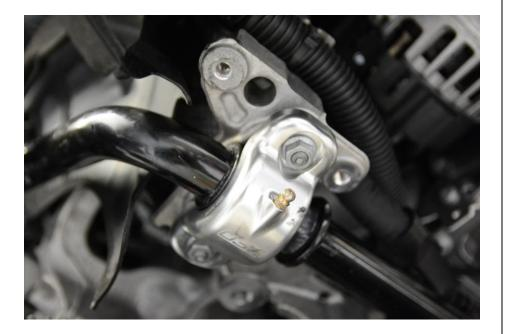
**Tip:** Orient brackets with zerk fittings facing forward for easy greasing.
