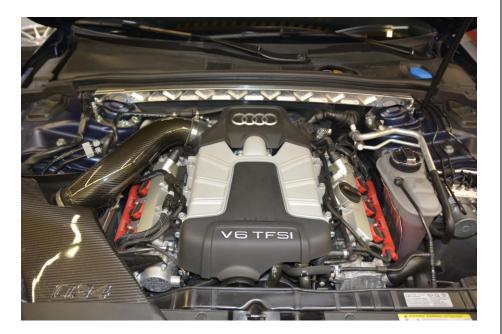
034Motorsport's Billet Strut Tower Brace for B8 Audi A4/S4/Allroad is the new standard in performance and durability. This brace was engineered with performance in mind, manufactured from billet aluminum for the optimum balance of strength vs. weight.
