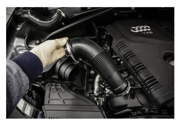
**Step 5** – Place supplied hose clamps over your 034Motorsport High Flow Silicone Turbo Inlet Hose, and leave loose to allow for some wiggle room when installing.
