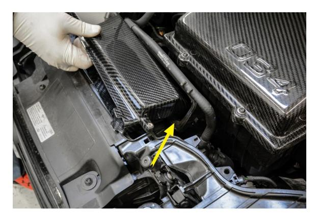
**Step 15 –** Once rear is inserted into airbox duct, slide forward snugly into core support.
