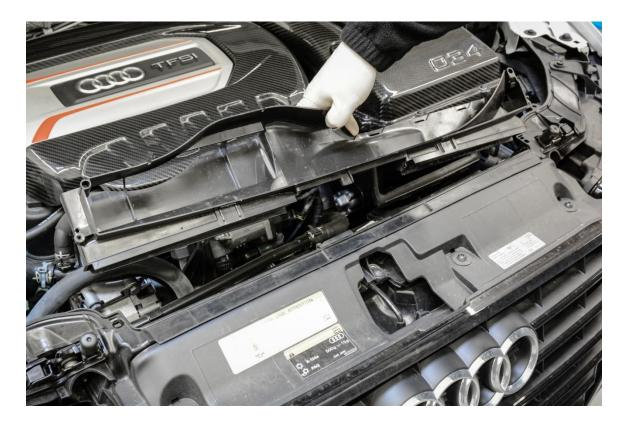
**Step 14 –** With your new 034Motorsport carbon fiber fresh air duct, insert rear portion into airbox duct first.
