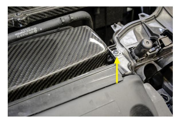
**Step 18 –** Using a 2mm Allen key, gently snug each M4 screw on either side of the duct. **Note: Careful not to overtighten!**
