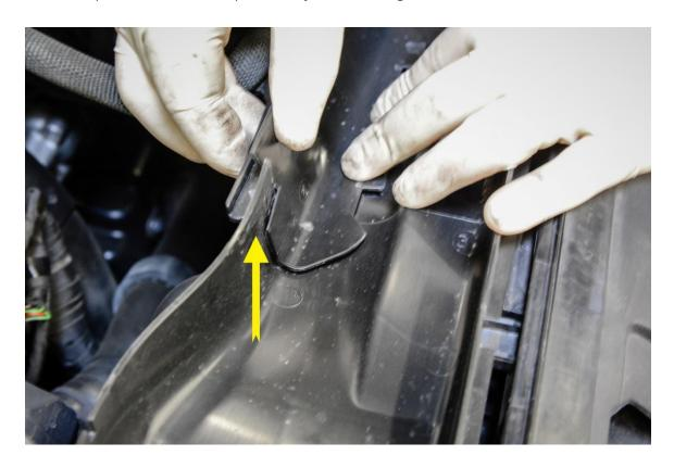
**Step 11** – Remove the rear portion of the duct completely from the engine bay.
