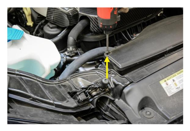
**Step 4** – Once the 2 bolts have been removed from the cover, locate and lift the clip on the back side of the air duct.
