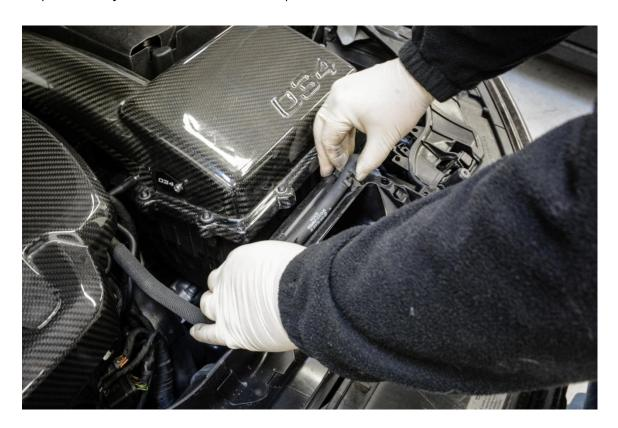
**Step 8** – Using a T25 Torx bit, remove the bolt securing each end of the fresh air duct to the radiator support. There will be 2 bolts total.
