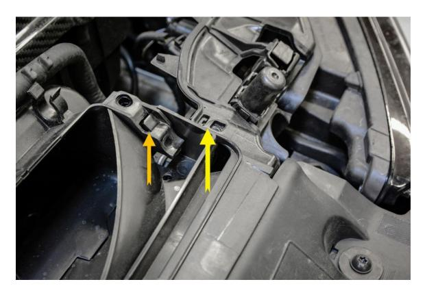
**Step 10** – Lift the rear portion of the duct up and away from the ridge of the main fresh air duct.
