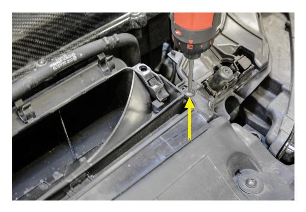
**Step 9** – With the bolts removed (see yellow arrow), push in the clip securing the rear duct to the main portion (see orange arrow).
