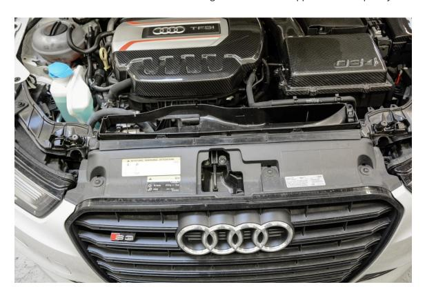
**Step 7** – Unclip the factory rubber hose from the 2 clips on the back side of the fresh air duct.
