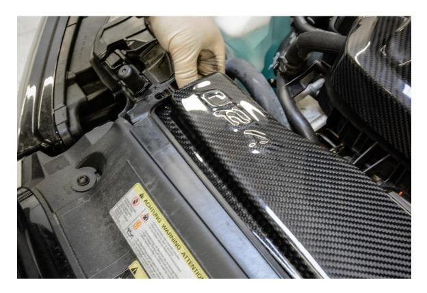
**Step 16** – Ensure the holes line up from the 034Motorsport carbon fiber fresh air duct and the core support mounting holes.
