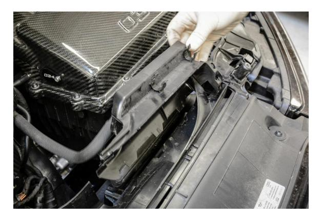
**Step 12 –** Using a flathead screwdriver, push the clip in on either side of the air duct securing it to the radiator support, and slide the duct back.
