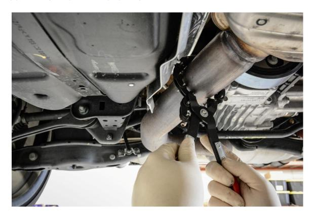
**Step 6** – Check that you've cut completely around the pipe. It should look similar to the image below.
