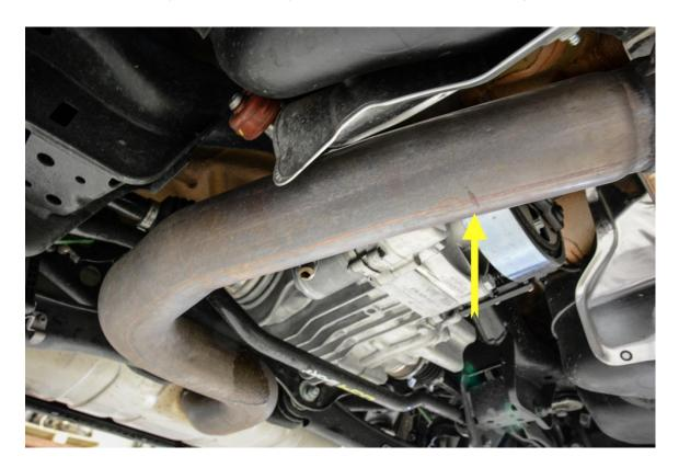
**Step 4** – We found the best way to cut the factory exhaust behind the resonator was using a pipe cutter. These can be found at most hardware stores.
