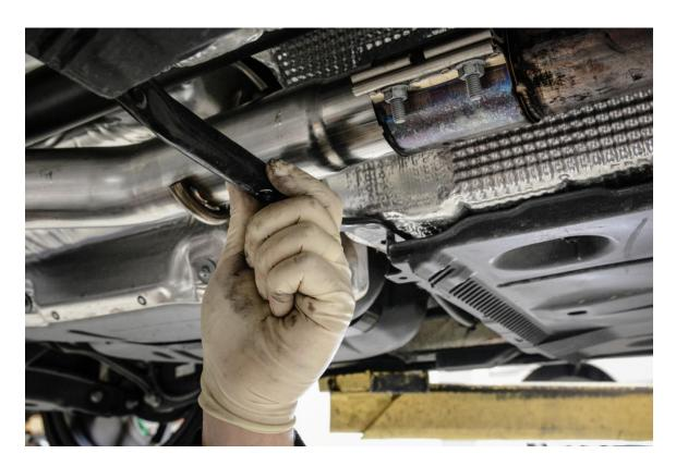
**Step 20 –** Check that exhaust clamps are secure. Lower vehicle from jackstands or lift, and enjoy the new roar of your 2.0T Gen 3!
