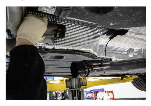
**Step 11** – Ensure that the cut made to the factory exhaust behind the resonator is complete. If so, the resonator should now be free and removed from the car. Remove existing factory exhaust clamp from downpipe.
