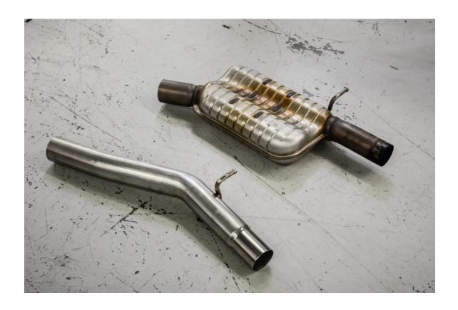
**Step 13** – Remove the factory exhaust hanger and bracket from the resonator, and transfer to 034Motorsport Res-X Resonator Delete. Preinstall one of the supplied exhaust clamps on rear portion of the 034Motorsport Res-X Resonator Delete.
