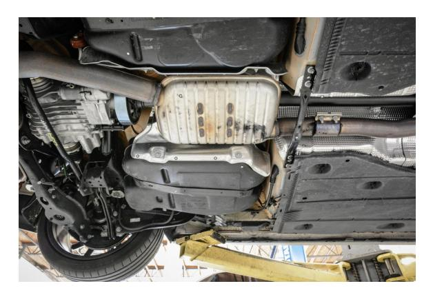
**Step 2** – Line up the 034Motorsport Res-X Resonator Delete underneath the factory resonator. Once aligned, mark the end of the 034Motorsport Res-X Resonator Delete on the factory exhaust with a pen.
