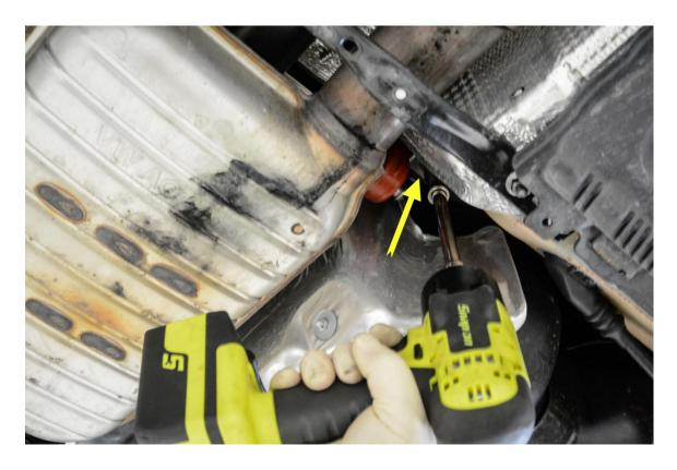
**Step 9** – Using a 13mm Socket, remove the 4 nuts securing the tunnel brace to the chassis and put the brace to the side.
