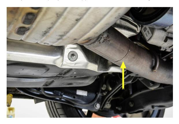
**Step 7** – Using a 13mm Socket, loosen the 2 nuts on the factory exhaust butt clamp before the resonator.
