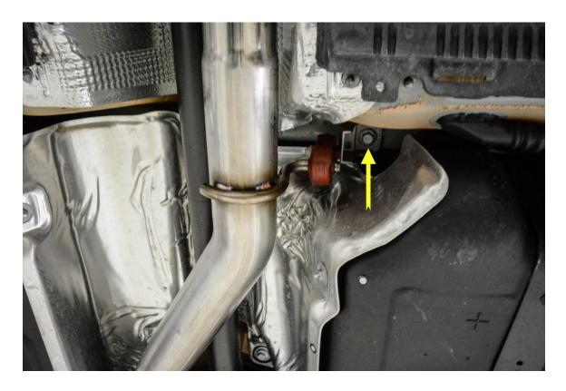
**Step 17 –** Using a 15mm Socket, tighten the 2 nuts on the exhaust clamp securing the front portion of the 034Motorsport Res-X Resonator Delete to the factory exhaust.
