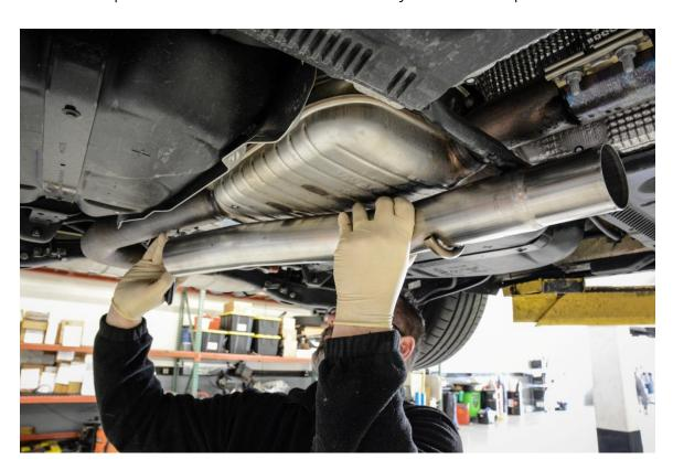
**Step 3** – This mark will be where you cut the factory resonator from the rear exhaust portion.
