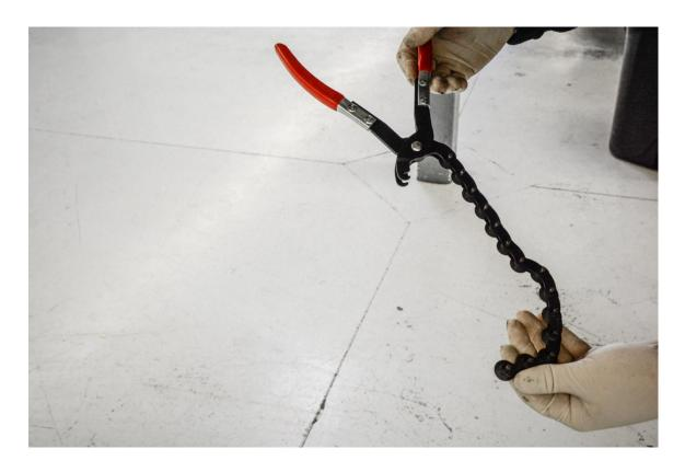
**Step 5** –Line up the pipe cutter over the factory exhaust along the line you just made. **Tip:** Double check that you're cutting the pipe as straight as possible for proper alignment.
