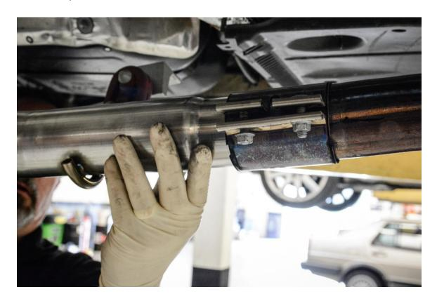
**Step 15** – Line up the rear exhaust with 034Motorsport Res-X Resonator Delete, and slide exhaust clamp back to join the two sections.
