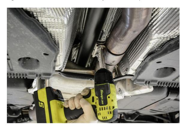
**Step 8** – Using a 13mm Socket, remove the bolt securing the exhaust hanger to the chassis.
