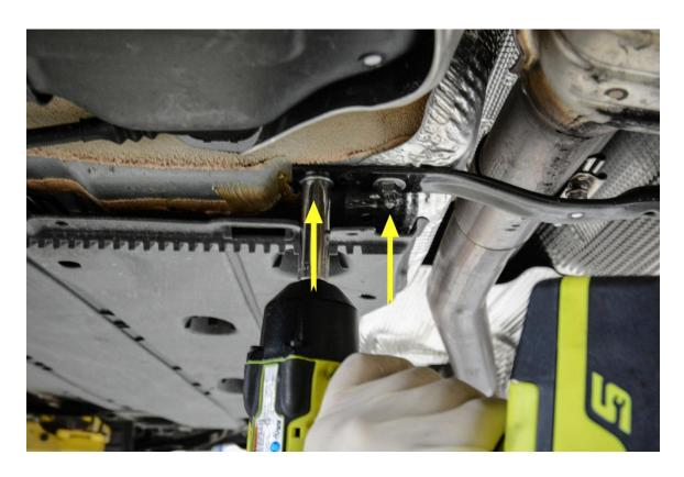
**Step 10** – Slide the factory exhaust butt clamp forward and out of the way. The front of the resonator should now be free from the downpipe.
