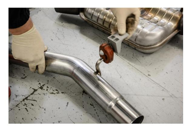
**Step 14 –** Slide one of the supplied exhaust clamps onto factory downpipe loosely. Then slide 034Motorsport Res-X Resonator Delete into front section of the factory exhaust. Ensure the clamp is covering equal amounts of factory exhaust and 034Motorsport Res-X Resonator Delete.
