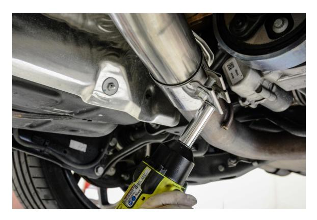
**Step 19 –** Reinstall the factory tunnel brace and install the 4 nuts securing brace to chassis with a 13mm Socket. Torque nuts to **20 Nm**.
