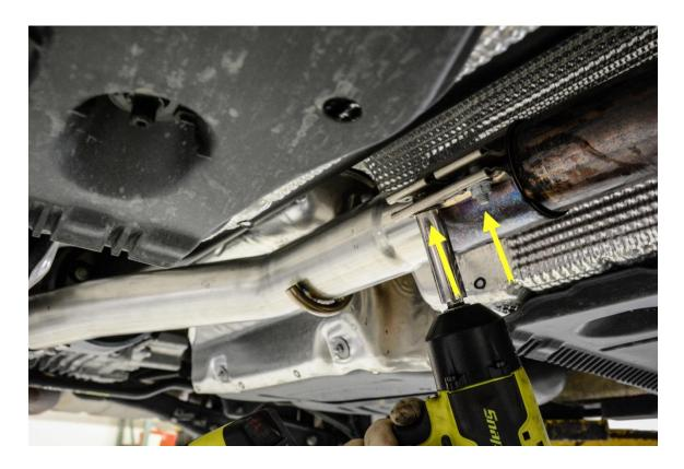
**Step 18 – Tip:** Rotate exhaust clamp to leave clearance for the rear differential. Once in place, use a 15mm Socket to tighten the 2 nuts securing the exhaust clamp to 034Motorsport Res-X Resonator Delete and rear portion of exhaust.
