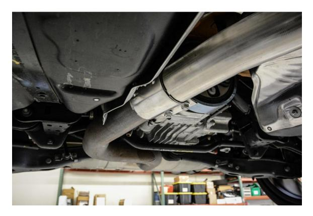
**Step 16 –** Using a 13mm Socket, install the bolt securing the exhaust hanger bracket to the chassis. Torque to **20 Nm**.
