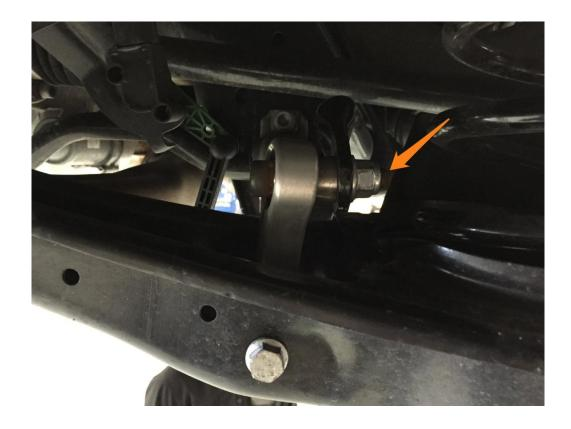
Step 8 – With the sway bar properly aligned, install the supplied Billet Aluminum Sway Bar Mounts with the zerk fitting pointing down. Secure using the supplied M8 Bolts & Washers. Torque to 28 Nm.
