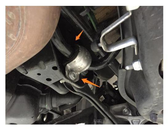
Step 3 – Using a 16mm wrench and 6mm triple square, remove the nut securing each of the rear sway bar end links to the rear sway bar.
