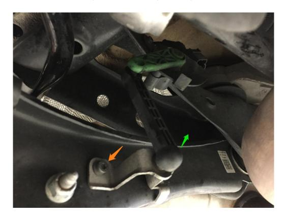
Step 6 – Preinstall the supplied Polyurethane Sway Bar Bushings onto your 034Motorsport Solid Rear Sway Bar Upgrade as shown below. Carefully install the 034Motorsport Solid Rear Sway Bar.
