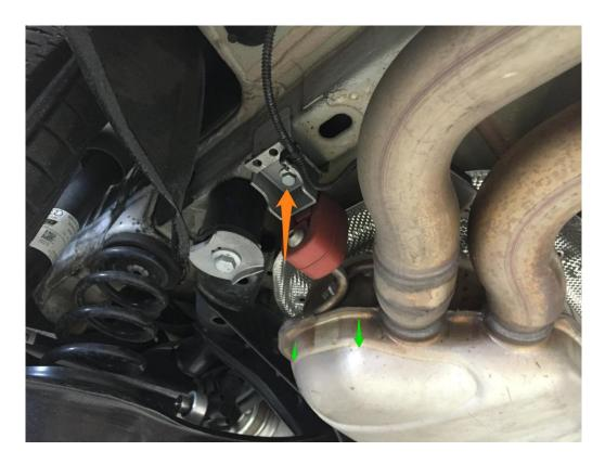
Step 5 – (Optional) In order to give yourself more room to work with, remove the T25 screws attaching the level sensor to the lower control arm. Carefully remove the factory rear sway bar.
