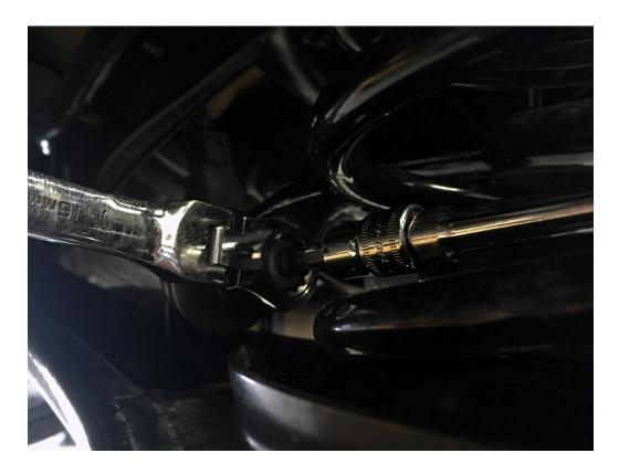
Step 4 – In order to remove the factory rear sway bar, you will need to lower the rear exhaust section. Using a 13mm wrench or socket, unbolt the two exhaust hangers on either side of the rear muffler. Support the exhaust if necessary.
