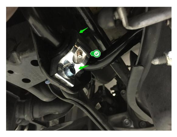
Step 9 – Verify that the Solid Rear Sway Bar is installed correctly, then (if you unbolted it) reinstall the level sensor bracket and level sensor to the lower control arm using the T25 screws.
