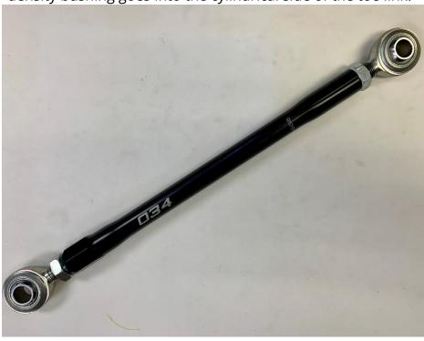
You are now ready to start the installation process. Use the length of the stock component as a starting point for the length of the 034 adjustable end links; expand or compress as best fits your needs
