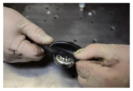
**Step 6**Insert machined steel adapters into heim joints.
