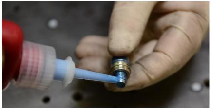
**Step 9**Install Allen bolts and spacers into heim joints.
