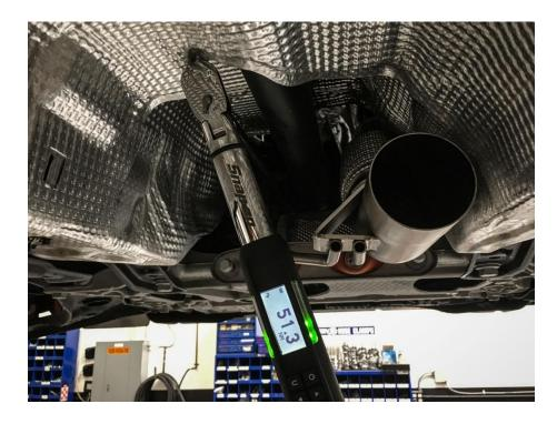
**Please Note:** We recommend replacing these bolts after removing. The part number for factory bolts is N90846102.
