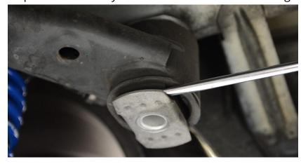
**Step 4**Remove the factory washer and set aside.
