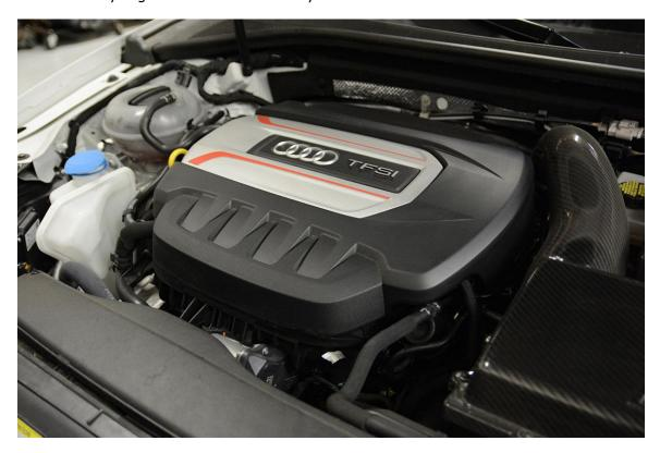
**Step 4** – Using a towel and isopropyl alcohol, thoroughly clean the factory Engine Cover.
