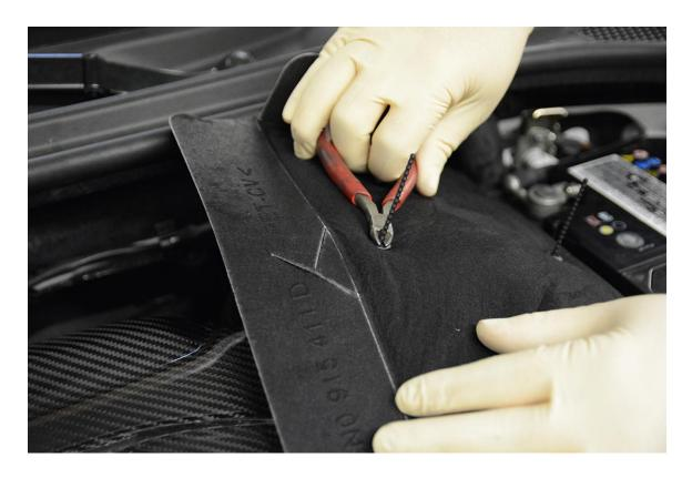
**Step 10** – Reinstall the battery blanket. Marvel at your work! Nap for ~6 hours or so.
