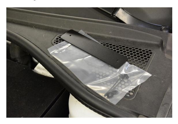
**Step 3** – Measure 5.125" from the back of the battery to position the supplied Powdercoated Steel Backing Plate correctly. **Important:** Measure from the back of the battery, not the back of the battery blanket!
