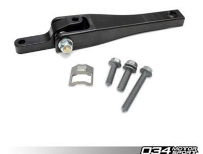
034Motorsport's Billet + Spherical Dogbone Mount and Upper Mount Insert for 8V/8S Audi A3/S3/TT/TTS & MkVII Volkswagen Golf/GTI/R is the new standard in performance and durability. This dogbone mount was engineered with performance in mind, manufactured from billet aluminum, and features a genuine Aurora Spherical Bearing to maintain proper articulation and reduce NVH transfer.
