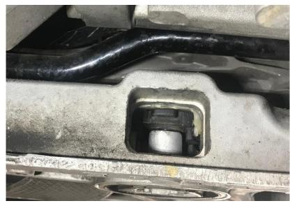
**Step 14**Reinstall the sway bar mounting bolts and torque to **28Nm**.
