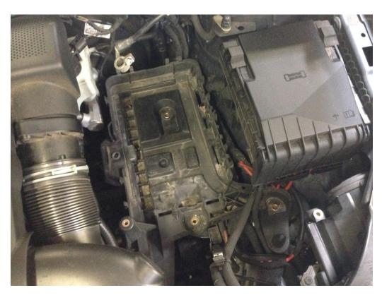
**Step 3** – At the fuse box, unbolt the left most wire – this should make the battery tray removal easier.
