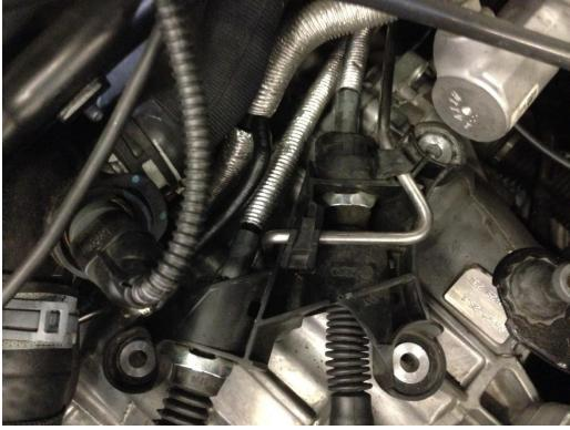
**Step 6** – Install the top half of the aluminum bushings, and reuse the stock mounting bolts. Tighten to 20 Nm.
