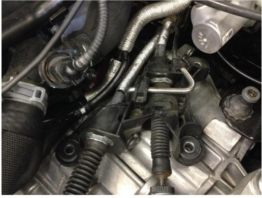
**Step 5** – Remove OEM rubber bushings and replace with 034Motorsport Billet Aluminum pieces. The larger part goes on the bottom, mating to the transmission.
