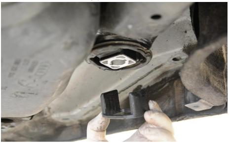
**Step 19** Apply silicone grease to the insert as pictured below.
