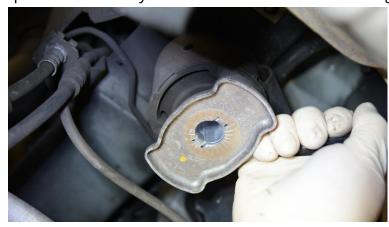
**Step 4**Remove the factory washer and set aside.
