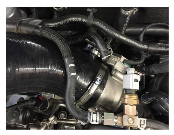
**Step 7** – Slip the other side onto the MAF housing at the intake. The airbox can be moved around to aid installation.
