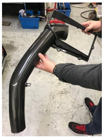
**Step 17** – Rotate intake tube within the airbox frame and install the air filter. Using an 8mm socket, tighten the hose clamp. **NOTE: Do not over-tighten**, as this may damage the carbon tube. It does not have to be very tight, just snug.
