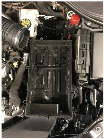
**Step 11** – The inlet pipe can now be removed. Disconnect the breather hose by pinching the connector and pulling away from the inlet pipe.
