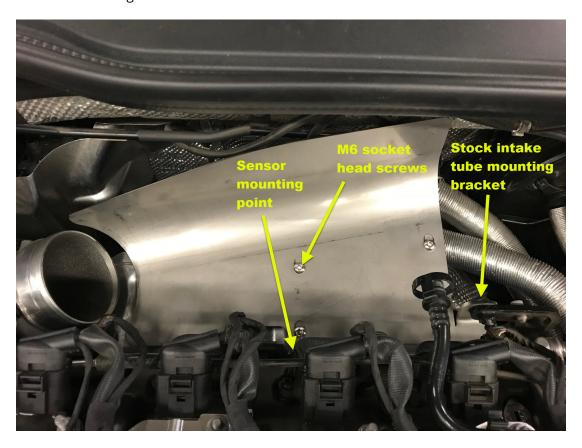
**Step 15 (2019+ vehicles)** – Using a 5mm Allen, remove the OE bypass hose from the throttle body by removing the two socket head screws (one top, one bottom).
