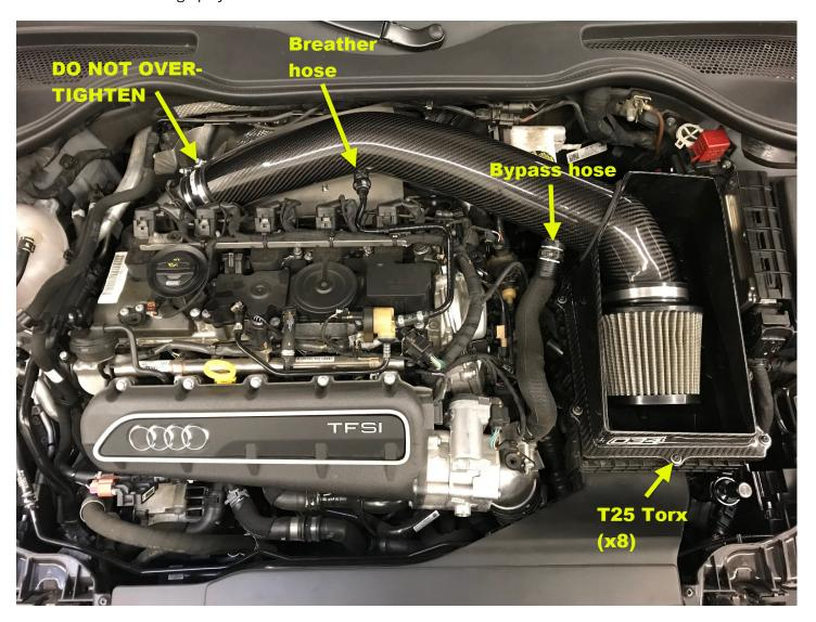
**Step 20 –** Connect breather hose (removed in step 11) to the intake tube fitting. It will snap on when fully seated (see image in Step 19).
