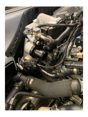
**Step 15** – Install silicone coupler to turbo inlet. Tighten hose clamp with 7mm socket.
