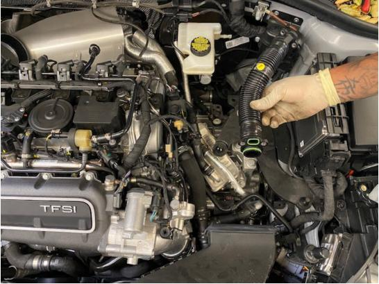
**Step 16 (2019+ vehicles)** – Install the small o-ring into the 034 adapter.
