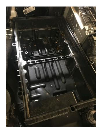
**Step 10** – Using the supplied hobby saw, remove the OE air filter center support.
