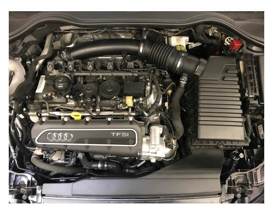
**Step 3** – Using a pair of pliers, loosen the spring clamp on the bypass hose and disconnect hose from OE intake. (For 2019+ vehicles, use a 5mm Allen to disconnect the bypass hose from the OE intake tube by removing the two Allen bolts.)
