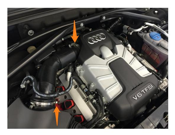
**Step 5** – Remove the factory throttle body hose.
