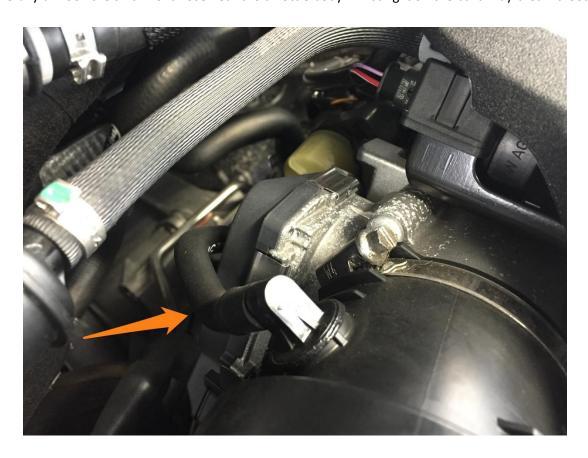
**Step 4** – Using a hose clamp driver or flathead screwdriver, loosen the factory worm clamps at the throttle body and the airbox.
