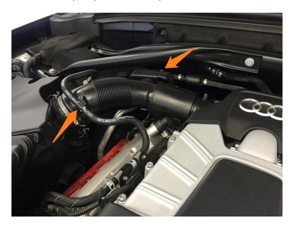
**Step 3** – Carefully unhook the small vent hose near the throttle body. Twisting it on the barb may break it loose.
