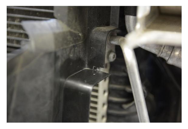
**Step 29 –** Remove backing from double sided tape and install air deflector plate, pressing firmly to attach tape.
