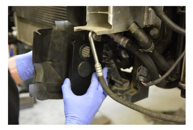
Step 30 – (B8 only) - Make a small notch in passenger side stock air deflector.
