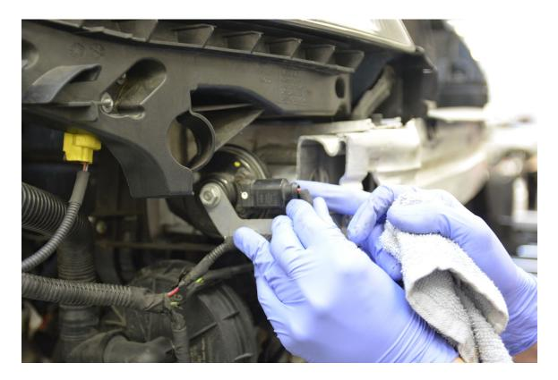
**Step 10** – Disconnect outside air temp sensor from plastic bracket. Be careful, bracket can be brittle.
