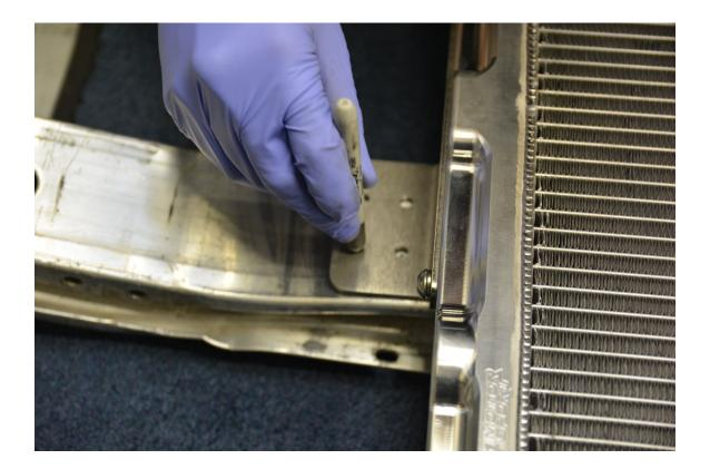
**Step 21 –** Using a center punch, mark center of each mark from step 20. This will make drilling much easier.
