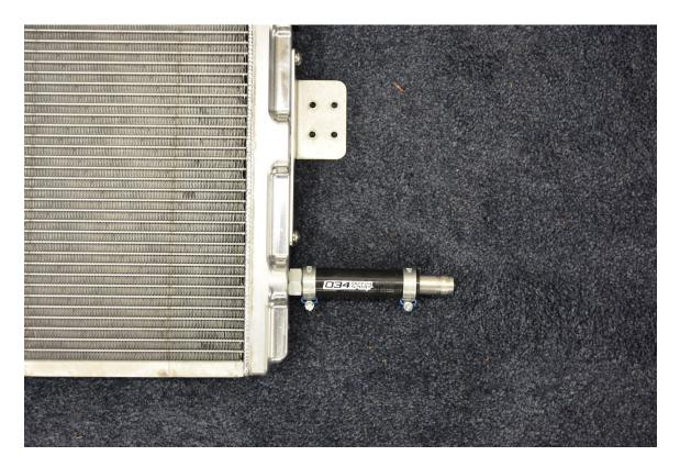
**Step 34** – Install heat exchanger assembly. Run silicone hoses through grommets in air deflector plates, and connect to stock lines.
