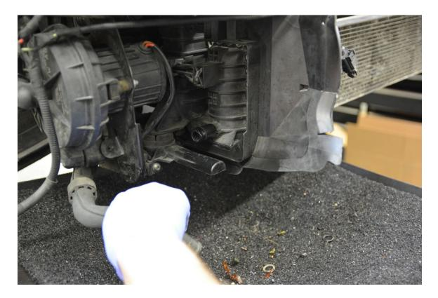
**Step 4** – Placing a suitable catch pan underneath, remove upper heat exchanger hose using pliers, or spring clamp pliers.
