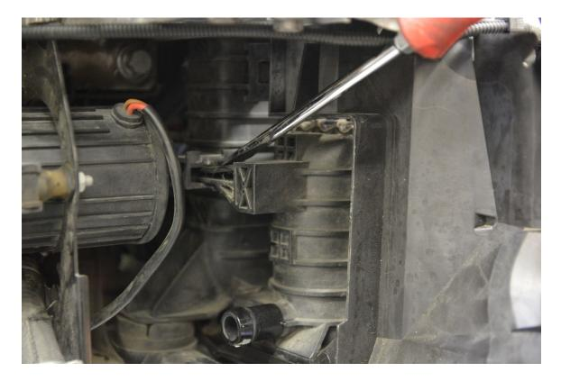
**Step 7** – Remove factory heat exchanger, careful not to damage factory plastic air ducts.
