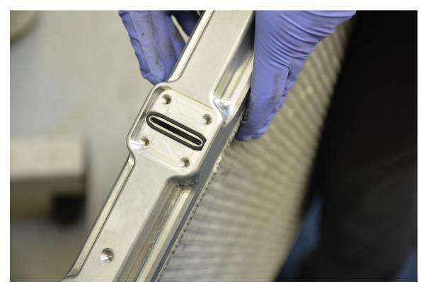
Step 15a (B8.5 only) – Insert diverter plate in driver side (LHD cars) end tank to create dual-pass unit.
