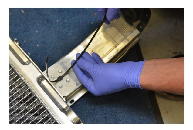
**Step 27 –** Assemble air block-off plates.
