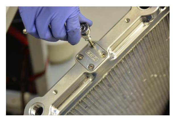
**Step 17** – Install -10AN plugs. **NOTE:** B8 will have a plug on each end; top on passenger side, bottom on driver side (LHD cars). B8.5 will have both plugs on passenger side, like in photo.
