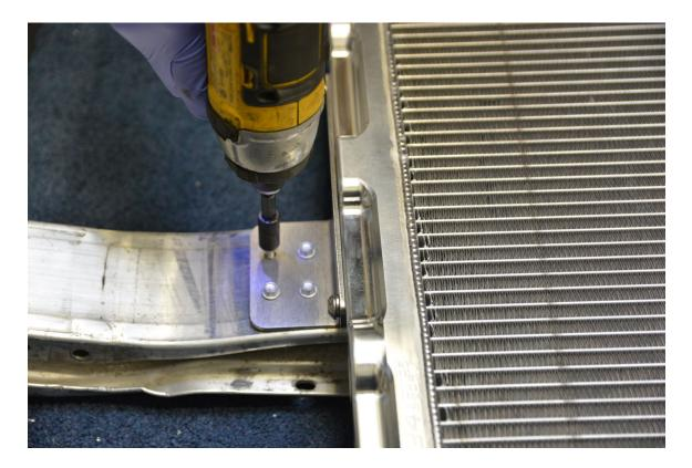
**Step 24 –** Drill 3/16" hole through bumper bar for zip-tie anchor.
