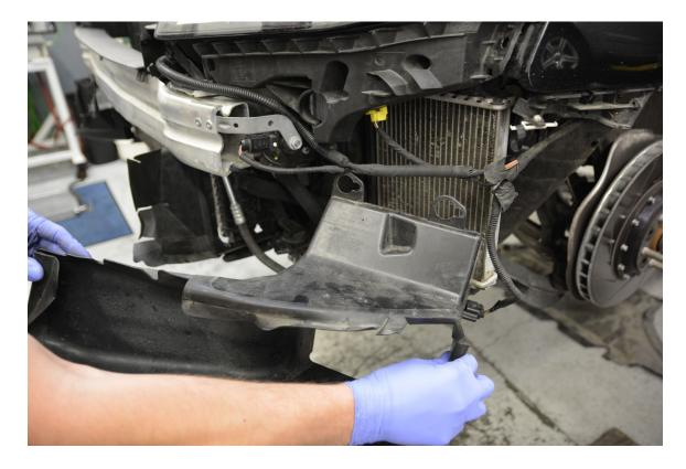
**Step 3** – Placing a suitable catch pan underneath, remove lower heat exchanger hose using pliers, or spring clamp pliers.
