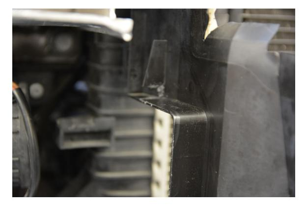
**Step 31 –** Remove backing from double sided tape and install air deflector plate, pressing firmly to attach tape.
