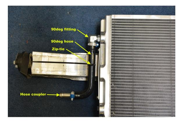
**Step 33** – Install straight fitting, hose and hose coupler.
