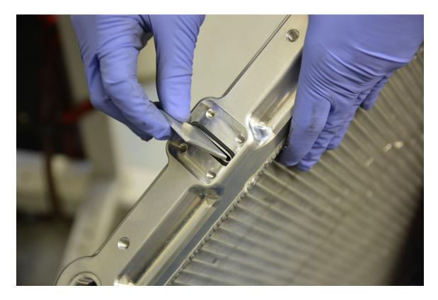
Step 15b (B8.5 only) –Diverter plate installed (driver side for LHD cars).
