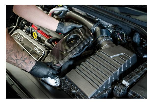
**Step 3** – Using a pair of pliers, loosen the spring clamp on the bypass hose and remove hose from OE intake.
