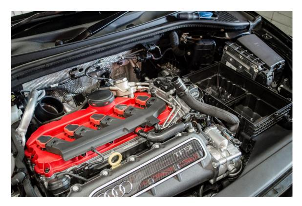
**Step 9** – Place 034Motorsport X34 Carbon Fiber Cold Air Intake System over factory lower airbox and align inlet tube with turbo inlet. **Note 1:** Be mindful of clearance around the HPFP. This can be slightly adjusted by rotating the inlet tube. **Note 2:** Loosely pre-install hose clamp on inlet pipe for easier installation once in place.
