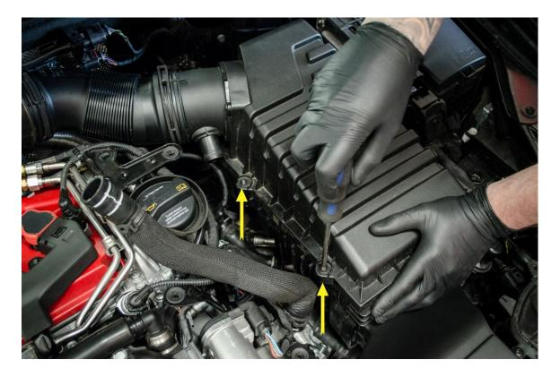
**Step 8** – The intake should now be completely free. Remove the factory intake from the car by simply lifting up and away. Remove the factory panel air filter from the lower air box and snow grate (if installed).
