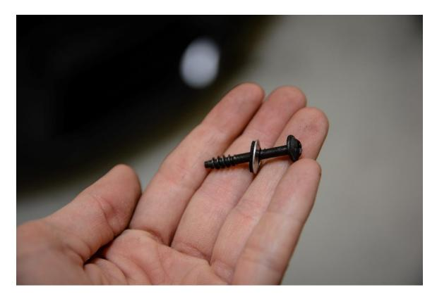
**Step 11** – Loosely install 7 of the factory airbox mounting screws with supplied neoprene washers, securing the heat shield to the lower factory airbox.
