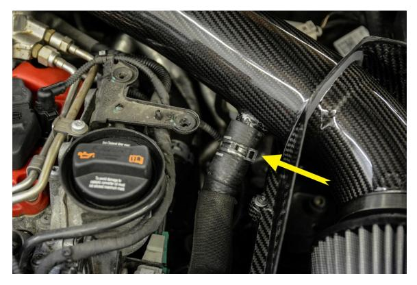
**Step 15** – Using those 2 opposable thumbs again, reinstall the factory carbon fiber trim around the oil fill cap.
