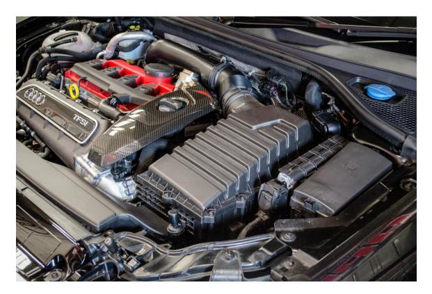
**Step 2** – Using your 2 opposable thumbs, remove the carbon fiber engine trim surrounding the oil filler cap.
