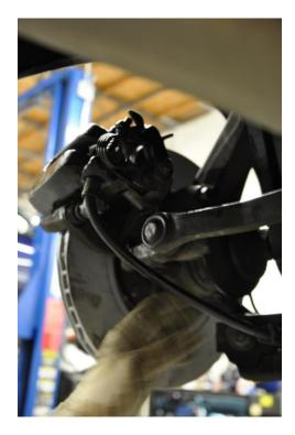
**Step 11** – Install the provided brake line adapter and install it onto the factory line using an 18mm wrench and 11mm wrench.
