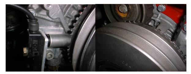
• The pulley should be torque'd to factory specifications, it can be painted as preferred, or else light surface rust will occur. It is *not recommended* to powder coat the pulley as the heat involved can weaken the dampening rubber.
