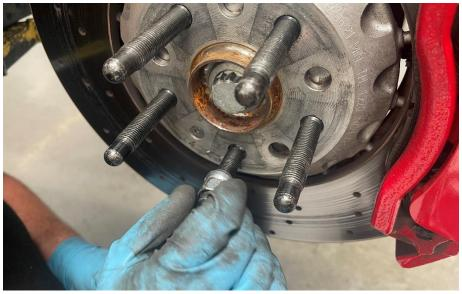
**Step 6**Thread a second nut onto the stud.
