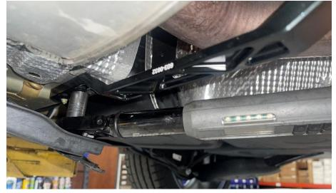
**Step 8** Using a 10mm socket, tighten the hardware for the belly pan, near the rear chassis brace.
