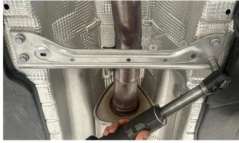
**Step 10** Remove the front chassis brace.
