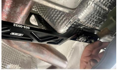
**Step 6** Using a 13mm socket, install the hardware to secure the factory chassis brace to the chassis.
