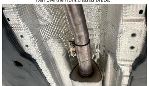
**Step 11** Using a 6mm Allen bit, install the front chassis brace with the provided hardware.
