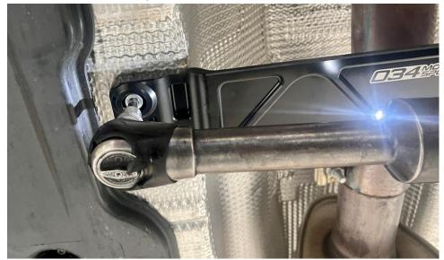
**Step 12** Torque the hardware to **20Nm.**
