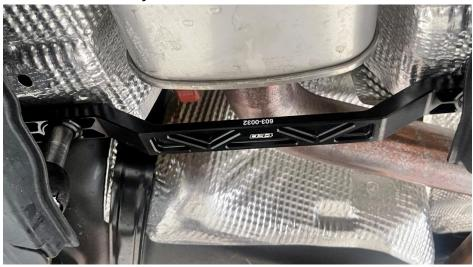
**Step 7** Torque the hardware to **20Nm.**
