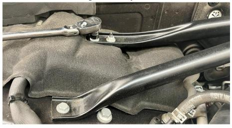
**Step 3**Using a 10mm socket, remove the nuts from the firewall
