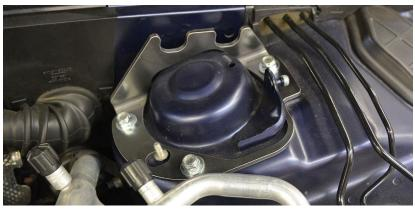
\*Some vehicles (S5's, late B8.5 S4's) do not have these treaded bosses on the right hand side strut tower. In this situation an additional hole (or two) will need to be drilled. If you are missing these bosses, an additional hole at Boss #1 is required. Doing so at Boss #2 is optional. Additional M8 bolts are included in the kit for this situation\*
