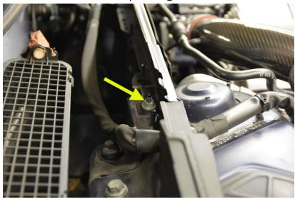
**Step 8**Lift cross brace off mounting points.
