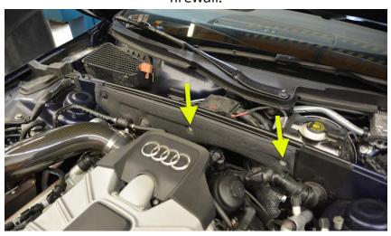
**Step 6**Remove 13mm nut on driver side of cross brace.
