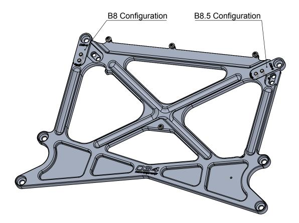
Set up the brace in the correct configuration for your vehicle prior to installation. Using red thread locker, tighten M10 hardware to 50 ft-lbs.
