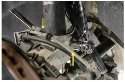
**Step 20**Using 12mm socket, torque upper 3 strut bolts to **30Nm**.
