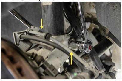
**Step 20**Using 12mm socket, torque upper 3 strut bolts to **30Nm**.
