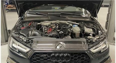
**Step 3**Unclip the coolant line from the reservoir.
