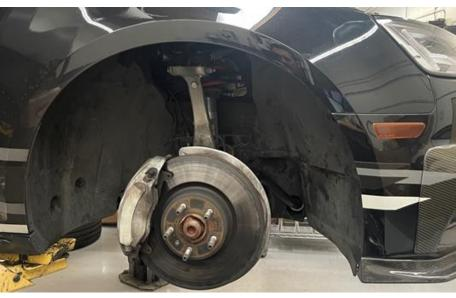
**Step 8**Using a 10mm socket, remove the plastic axle guard.
